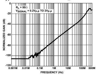
FIGURE 18. OFF-ISOLATION AUDIO SWITCHES
