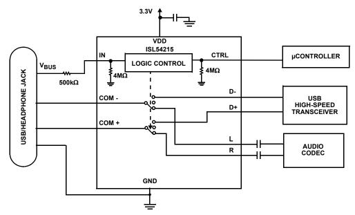
FIGURE 9. LOGIC CONTROL VIA  $V_{\mbox{\scriptsize BUS}}$  VOLTAGE FROM COMPUTER OR USB HUB
