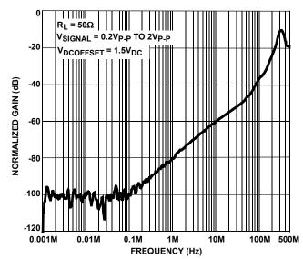
FIGURE 17. OFF-ISOLATION USB SWITCHES
