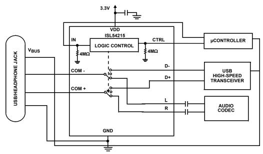
FIGURE 8. LOGIC CONTROL VIA MICROPROCESSOR
