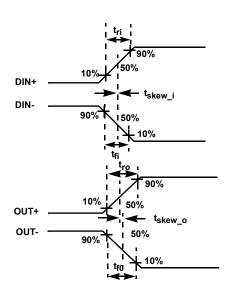
FIGURE 7A. MEASUREMENT POINTS
