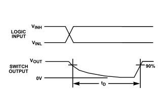
FIGURE 2A. MEASUREMENT POINTS
