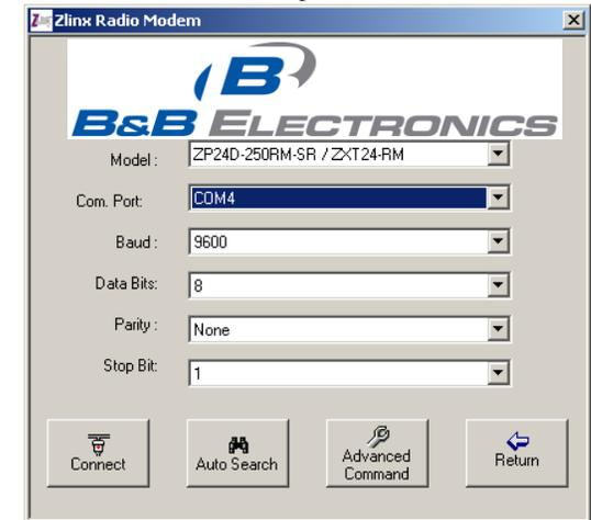
Figure 3. Communication Parameters Screen
