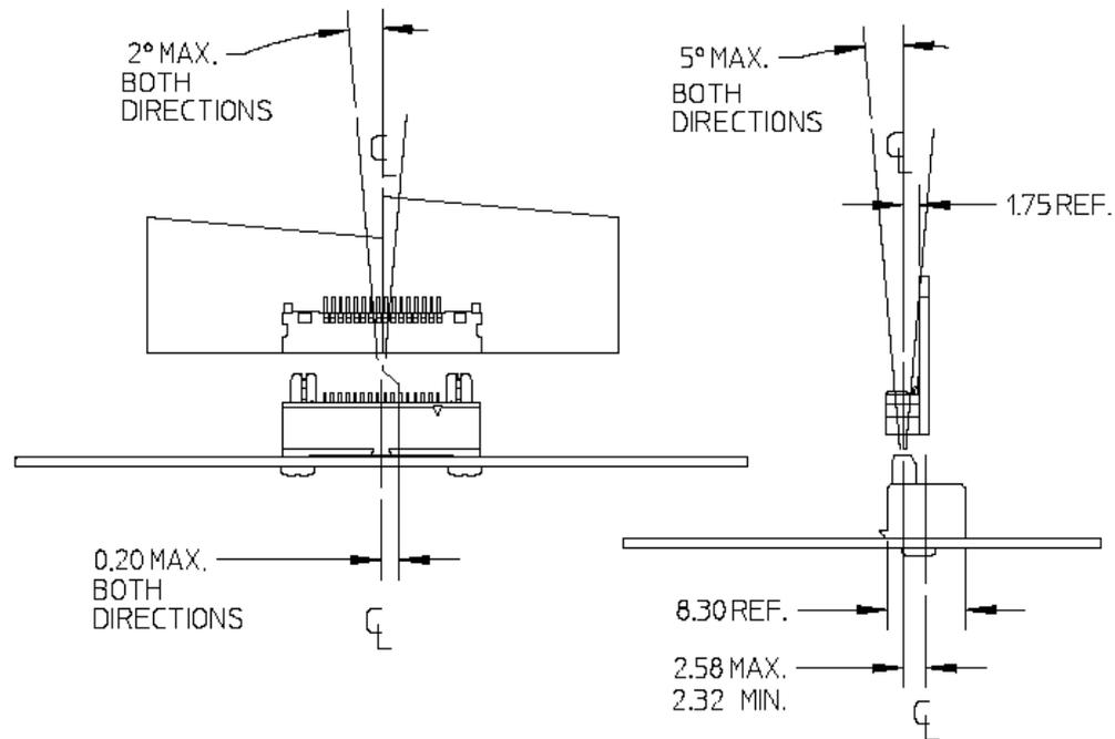
NOTE: Mating misalignment may significantly influence the long-term durability of the connectors. The risk of housing wear diminishes with increasing the accuracy of connector alignment.
