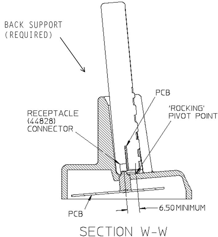
Figure 21. Section View of Shelf-Style Cradle (units: mm)
