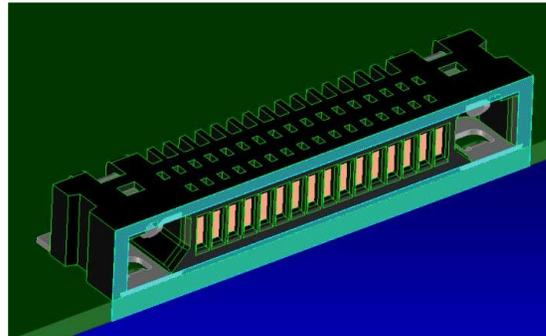
Gaskets may be applied to the top and sides, or front surfaces.
