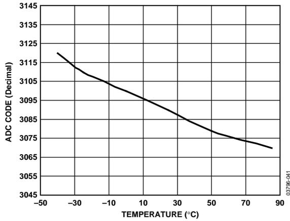
Figure 18. ADC Code vs. Temperature (2.7 V Supply)
