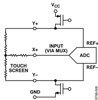
Figure 30. Ratiometric Conversion of Touch Screen Inputs
