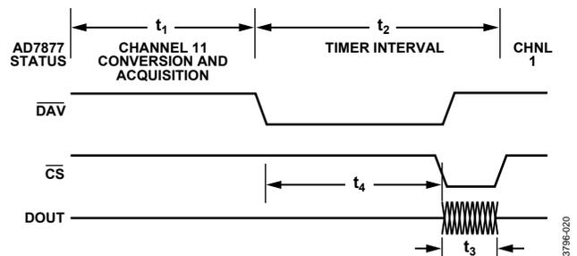
Figure 42. Timing for Reads after  $\overline{DAV}$  Goes Low
