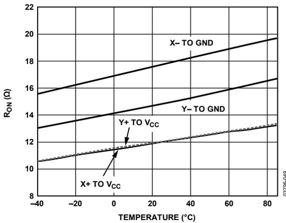
Figure 14. Switch On Resistance vs. Temperature
