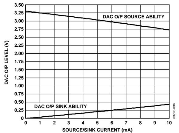
Figure 23. DAC Source and Sink Current Capability
