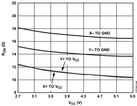
Figure 13. Switch On Resistance vs.  $V_{CC}$
