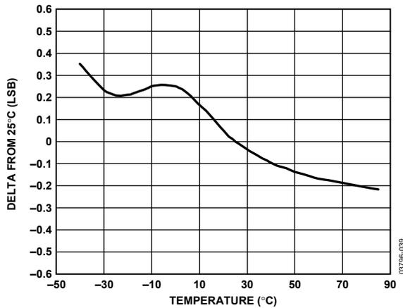
Figure 8. Change in ADC Gain vs. Temperature
