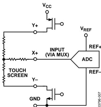
Figure 29. Single-Ended Conversion of Touch Screen Inputs
