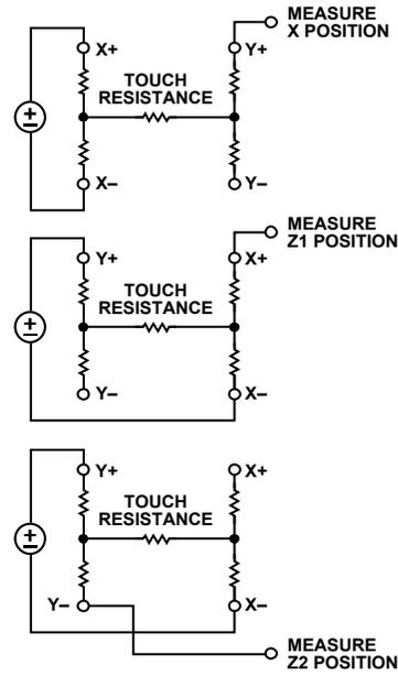
Figure 31. Three Measurements Required for Touch Pressure
