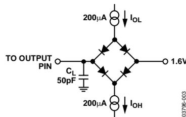
Figure 3. Load Circuit for Digital Output Timing Specifications
