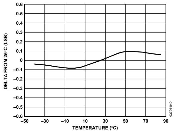
Figure 10. Change in ADC Offset vs. Temperature
