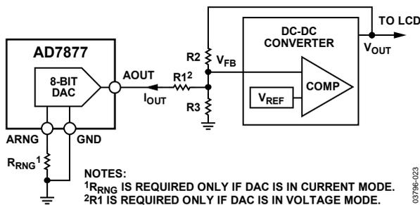
Figure 45. Using the DAC to Adjust LCD Contrast
