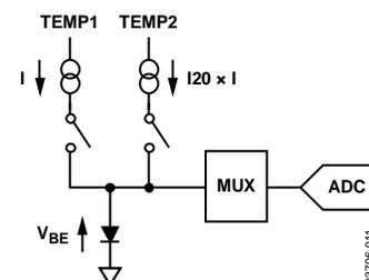
Figure 33. Block Diagram of Temperature Measurement Circuit
