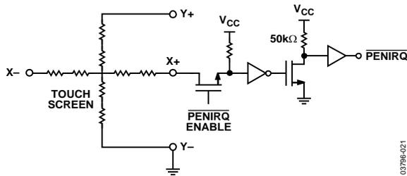
Figure 43.  $\overline{\text{PENIRQ}}$  Output Equivalent Circuit
