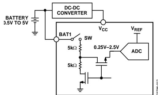
Figure 34. Block Diagram of Battery Measurement Circuit
