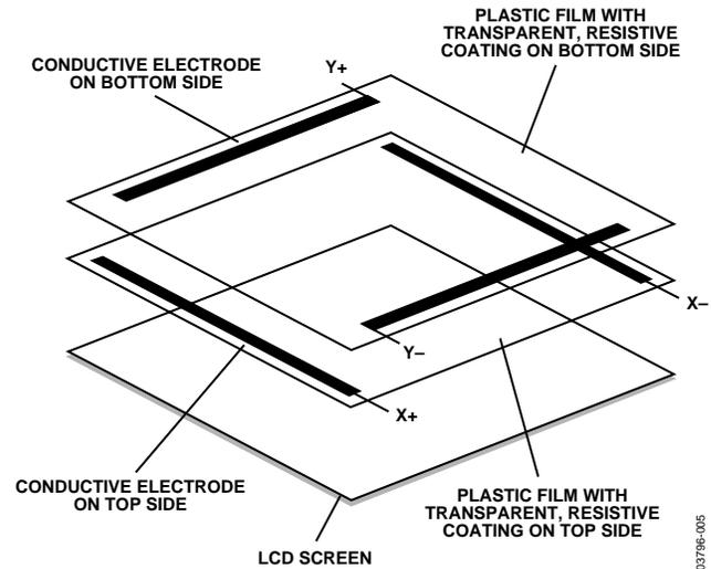
Figure 27. Basic Construction of a Touch Screen
