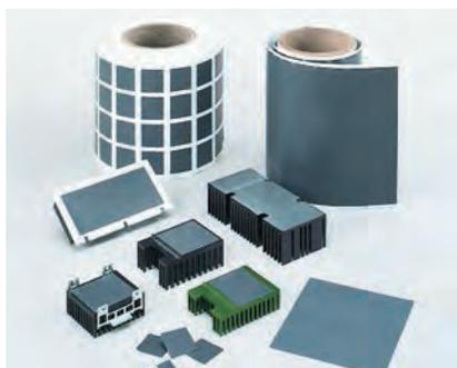
HI-FLOW 105 is a phase change material coated on both sides of an aluminum substrate. It is designed specifically to replace grease as a thermal interface, eliminating the mess, contamination and difficult handling associated with grease. HI-FLOW 105 is tack-free and scratch-resistant at room temperature, and does not require a protective liner in shipment when attached to a heat sink.
