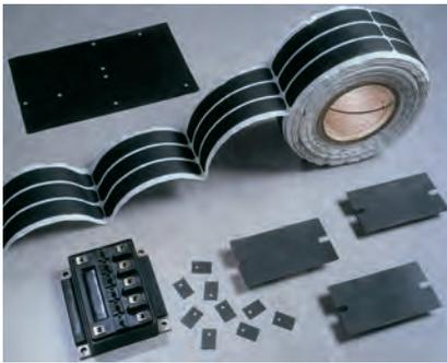
BERGQUIST Q-PAD 3 is a grease-only replacement that does away with contamination of electronic assemblies and reflow solder baths. Q-PAD 3 may be installed prior to soldering and cleaning with confidence. When clamped between two surfaces, the elastomer conforms to surface textures, thereby creating an air-free interface between heat-generating components and heat sinks.
