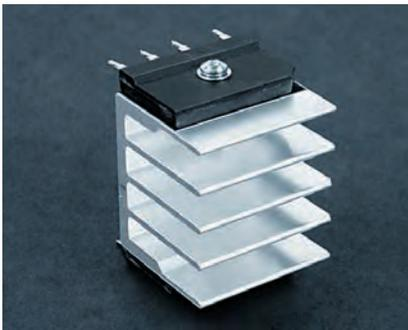
Q-PAD II is a composite of aluminum foil-coated on both sides with thermally/electrically conductive SIL PAD rubber. The material is designed for those applications in which maximum heat transfer is needed and electrical isolation is not required. Q-PAD II is the ideal thermal interface material to replace messy thermal grease compounds.
