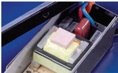
GAP PAD 1450 is a highly compliant GAP PAD material that is ideal for fragile component leads. The material includes a PEN film, which facilitates rework and improves puncture resistance and handling characteristics. The tacky side of GAP PAD 1450 maintains a conformable, yet elastic nature that provides excellent interfacing and wet-out characteristics, even to surfaces with high roughness or uneven topography.
