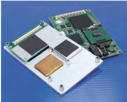
GAP PAD 1500 has an ideal filler blend that gives it a low-modulus characteristic which maintains optimal thermal performance yet still allows for easy handling. The natural tack on both sides of the material allows for good compliance to adjacent surfaces of components, minimizing interfacial resistance.
