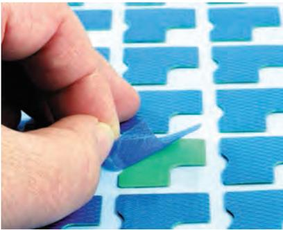
GAP PAD 1000SF is a thermally conductive, electrically insulating, silicone-free polymer specially designed for silicone-sensitive applications. The material is ideal for applications with high standoff and flatness tolerances. GAP PAD 1000SF is reinforced for easy material handling and added durability during assembly. The material is available with a protective liner on both sides of the material. The top side has reduced tack for ease of handling.
