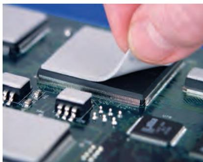
GAP PAD 2000S40 is recommended for low-stress applications that require a mid-to high-thermally conductive interface material. The highly conformable nature of the material allows the pad to fill in air voids and air gaps between PC boards and heat sinks or metal chassis with stepped topography, rough surfaces and high stack-up tolerances.
