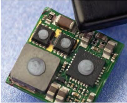
LIQUI-FORM 2000 is a high thermal conductivity liquid formable material designed for demanding applications requiring a balance between dispensability, low component stresses during assembly and ease of rework.
