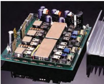
GAP PAD VO Soft is recommended for applications that require a minimum amount of pressure on components. GAP PAD VO Soft is a highly conformable, low-modulus, filled-silicone polymer on a rubber-coated fiberglass carrier. The material can be used as an interface where one side is in contact with a leaded device.
