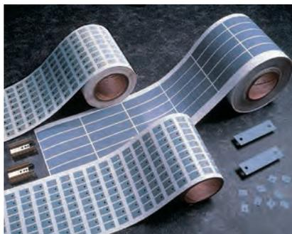
SIL PAD K-6 is a medium performance, film-based thermally conductive insulator. The film is coated with a silicone elastomer to deliver high performance and provide a continuous, physically strong dielectric barrier against “cut-through” and resultant assembly failures.
