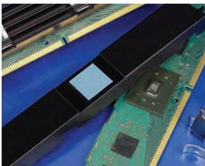
HI-FLOW 565UT is a naturally tacky, thermally conductive phase change material which is supplied in an easy to use tabulated pad form. In the application the material undergoes a phase change softening, starting near 52°C. The phase change softening feature improves handling characteristics prior to a facilitated assembly. At application temperatures and pressures, HI-FLOW 565UT wets out the thermal interfaces producing a very low thermal impedance.
