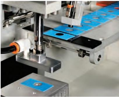
SIL PAD 1500ST (Soft Tack) is a fiberglass-reinforced thermal interface material that is naturally tacky on both sides. SIL PAD 1500ST exhibits exceptional thermal performance.
