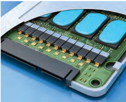
Gap Filler 4000 is a two-part, high performance, thermally conductive, liquid gap-filling material. The mixed material will cure at room temperature and can be accelerated with the addition of heat. Gap Filler 4000 offers an extended working time to allow greater flexibility in the customer's assembly process.
