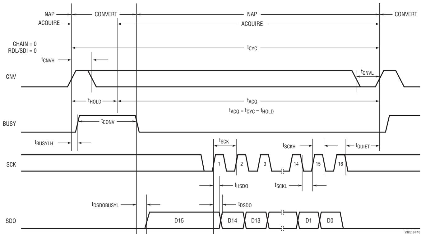
Figure 10. Using a Single LTC2326-16 in Normal Mode
