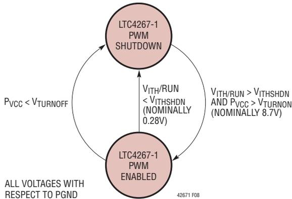
**Figure 8. LTC4267-1 Switching Regulator Start-Up/Shutdown State Diagram**
