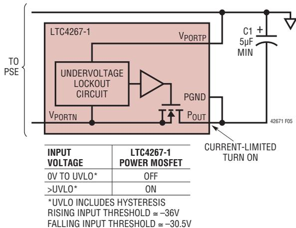
Figure 5. LTC4267-1 V<sub>PORTN</sub> Undervoltage Lockout
