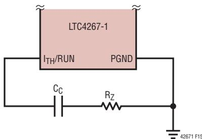
Figure 15. Main Loop Compensation for a Nonisolated Design
