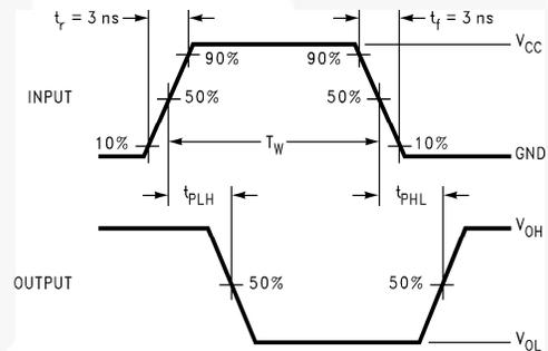
**Figure 5. AC Waveforms**
