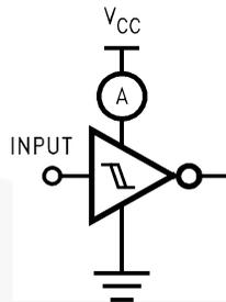
**Figure 6. I<sub>CCD</sub> Test Circuit**
