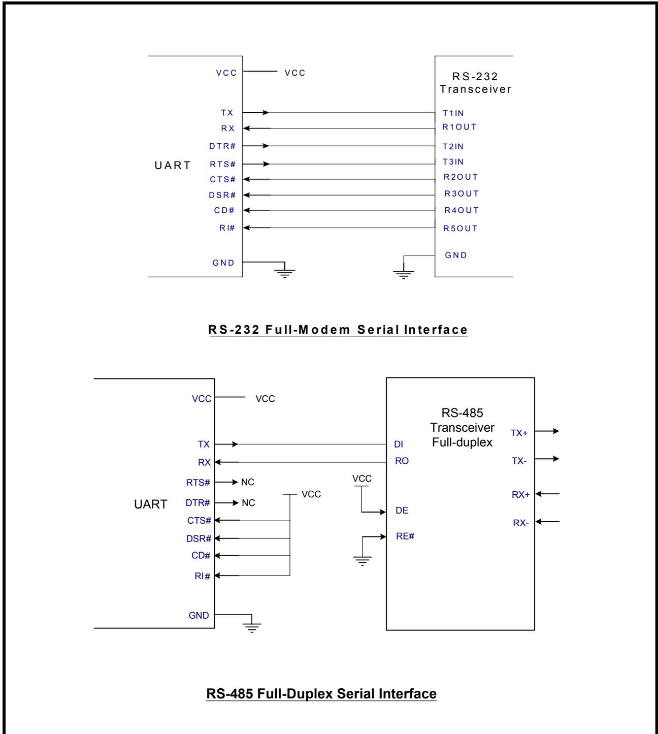
**FIGURE 5. XR16M581 TYPICAL SERIAL INTERFACE CONNECTIONS**
