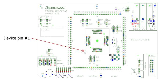
Figure 3 - RH850-F1X-100PIN-PB-T1-V3 top view
