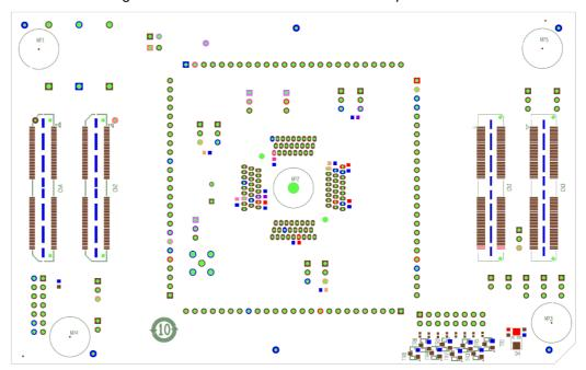
Figure 4 – RH850-F1X-100PIN-PB-T1-V3 bottom view
