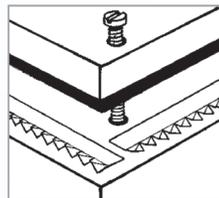
Adhesive-mounted beryllium copper contact strips with scientific twist design offer narrow electronic gaskets for general shielding applications.
