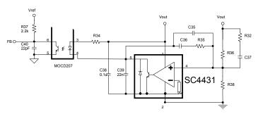
The signal at the FB pin is then compared to the 3X amplified signal from the current sense/ slope compensation CS pin. Matched out of phase signals are generated to control the OUTA and OUTB gate drives of the two phases. A single ramp signal is used to generate the control signals for both phases, hence achieving a tightly matched per phase operation.
