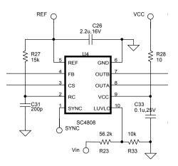
The oscillator has a ramp voltage of about Vref/2. The oscillator frequency is twice the frequency of the OUTA and OUTB gate drive controls.
