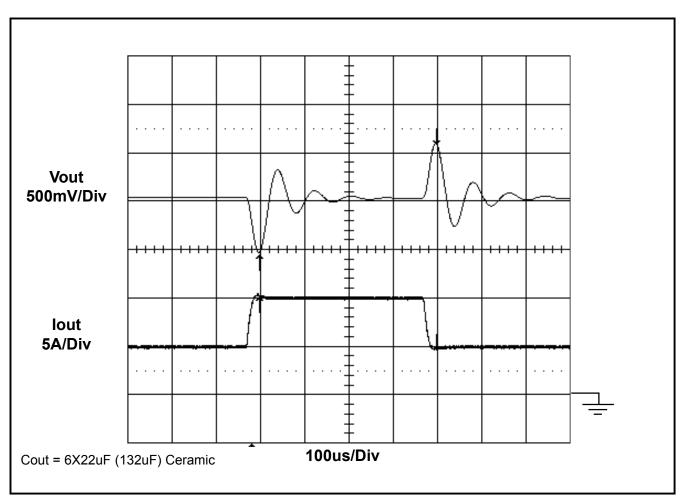
Typical SC4808C Push Pull Converter Step Load plot at Vin = 48V, Vout = 3.3V, Step = 37% to 75% lout, Fosc = 650kHz
