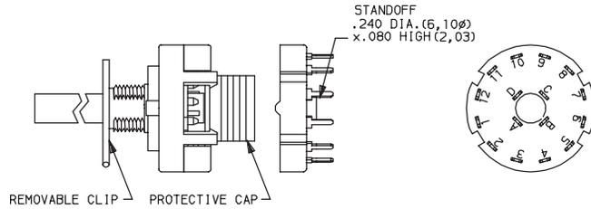
**NOTE:** Switches with 'C' or 'MC' terminations have additional terminal no. 9 as switch support only. This terminal is not connected electrically inside switch. Solder and clean switch base on PC board with other components, then snap on housing/actuator assembly. See page K-7 for installation instructions.
