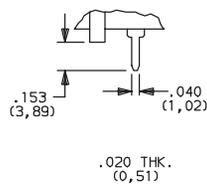
**MC** MODULAR BASE (for wave soldering)
