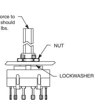
Install switch with stop ring (if used) and lockwasher in back of panel. Tighten hex nut from front of panel.
