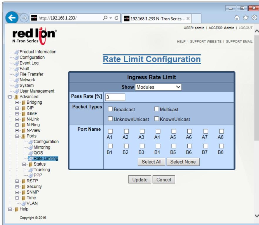
**Show:** View the ports that are available to install (Modules), currently installed or currently linked up.
