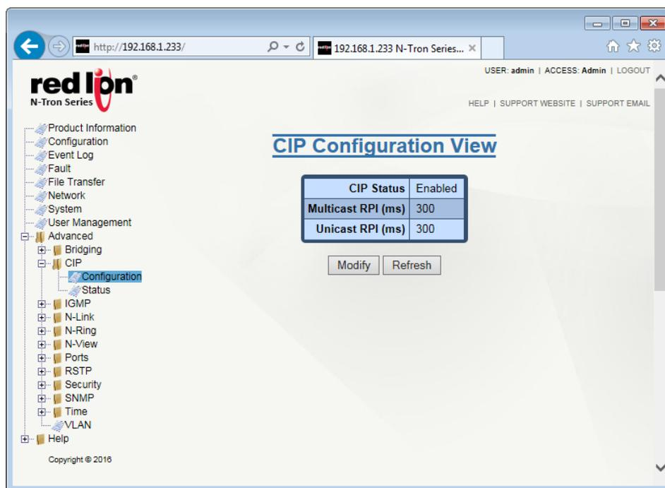
**CIP Status:** This field determines whether CIP is enabled or disabled on the NT24k switch. The default setting is Enabled.
