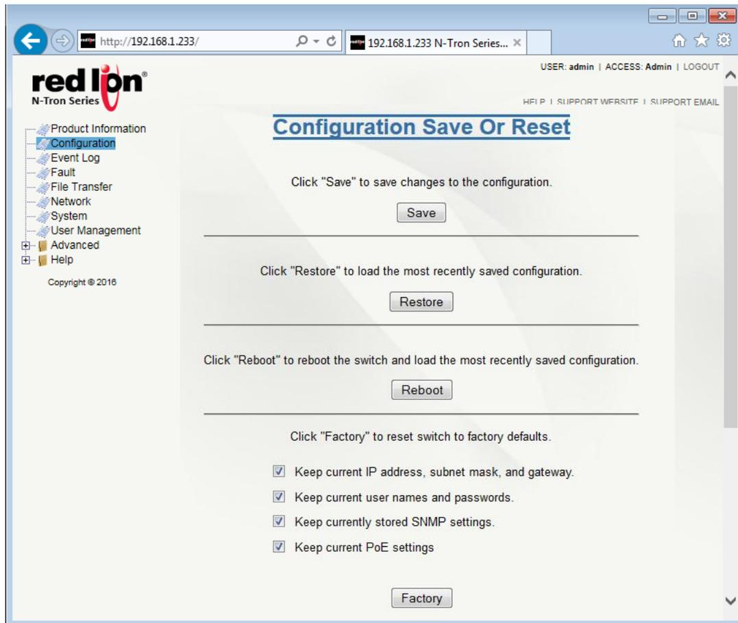
**Save:** Click on the *Save* button to save all current changes to the configuration stored in non-volatile memory for use after the next power cycle or reboot. If a configuration device is installed, the configuration will also be saved to the device. This option is only available when there is no misconfiguration.
