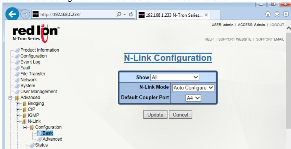
**Show:** View the ports that are available to install (Modules) currently installed or currently linked up.
