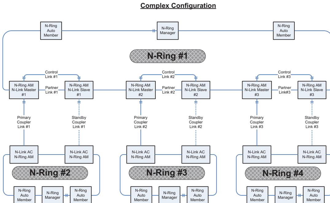
**Configuration steps to redundantly couple 2 N-Ring networks:**
