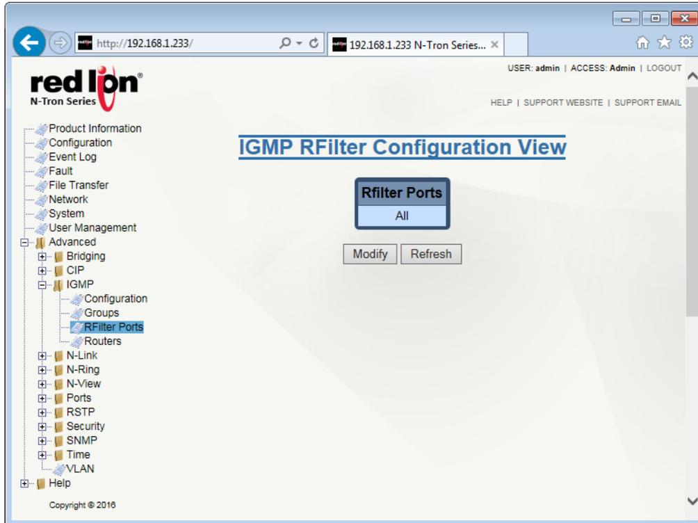
Known group multicast addresses are learned from dynamic IGMP Snooping operations. If IGMP is enabled and a port is a router port, then having RFilter enabled will stop IGMP group data from egressing on the port unless a join to that specific IGMP group has come into the port. IGMP controls (Join, Leave, Query) are still sent.
