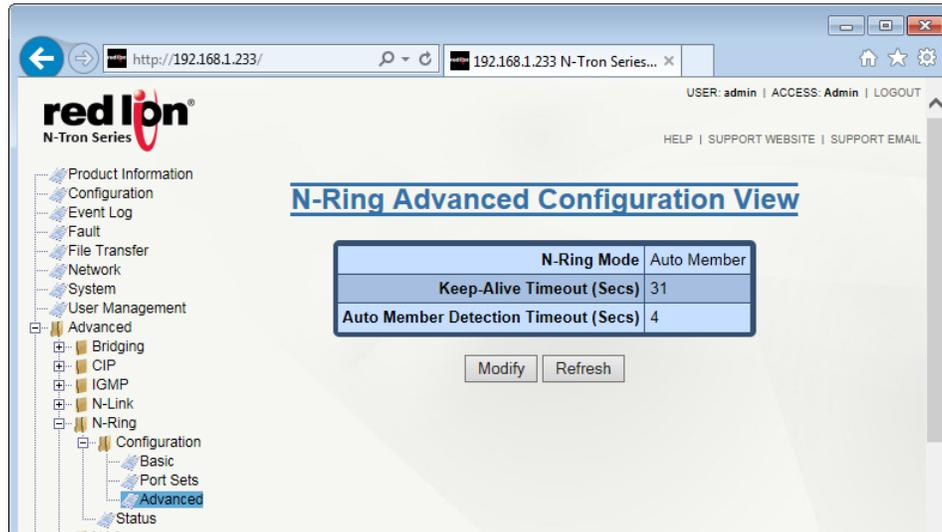
**N-Ring Mode:** This field is defined in the N-Ring/Configuration/Basic dialog window.
