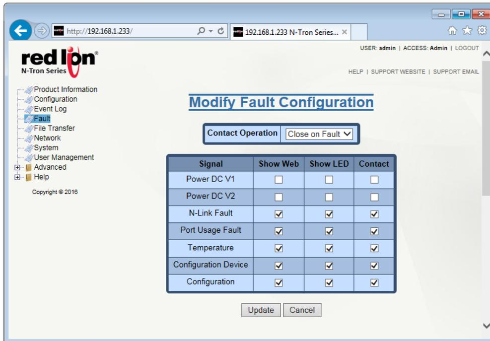
Select the desired notification settings and click on the *Update* button to save any changes. Once the save is complete, the dialog window will change to Fault Configuration.
