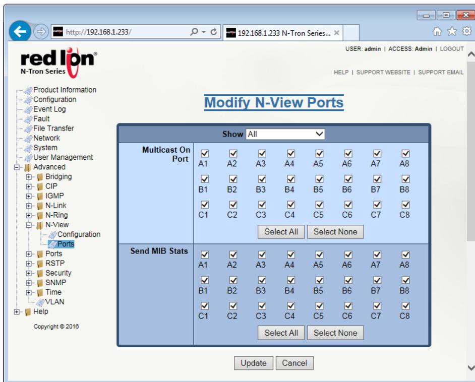
The user can modify these two variables to enable or disable N-View related multicast out of the port and if MIB stats are sent out for those ports. The ports that can be installed (Modules), currently installed or currently linked up can also be viewed.
