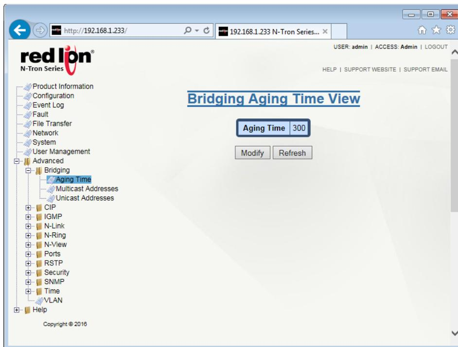
To modify the Aging Time field, click on the *Modify* button. Enter the desired Aging Time (value must be between 10 - 630 seconds) and click on the *Update* button. The default value for this field is 300 seconds. To save the changes made, return to the Configuration menu and click on the *Save* button.
