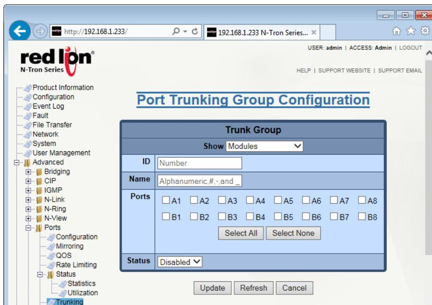
**Show:** View the ports that are available to install (Modules) currently installed or currently linked up.
