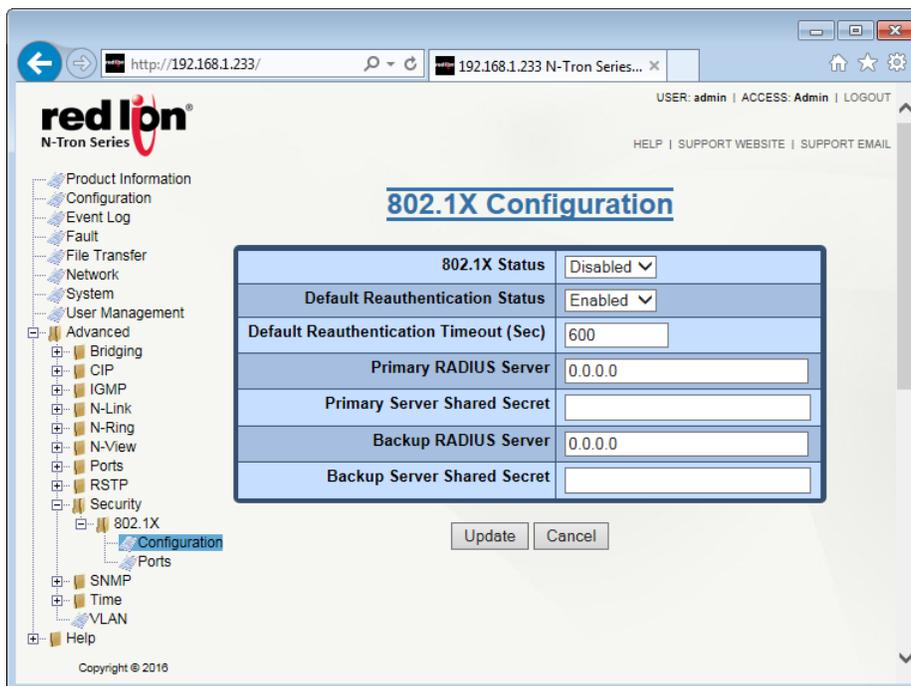
**802.1x Status:** This field indicates whether the 802.1x feature is enabled or disabled. At least one RADIUS server must be specified for 802.1x to be enabled. Ports must also be individually enabled on the ports configuration page.
