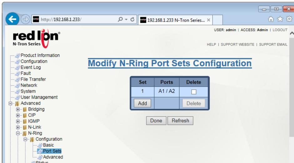
**N-Ring Ports:** A new port set can be added by selecting the N-Ring ports from the N-Ring Ports pull-down lists and clicking on the *Add* button.
