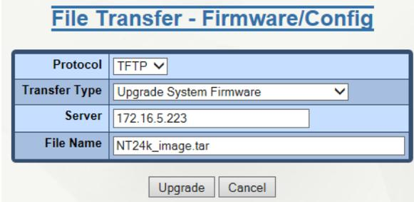
**Server:** This field displays the IP address of the TFTP server. It is automatically populated with the IP address of the PC which is connected to the switch.
