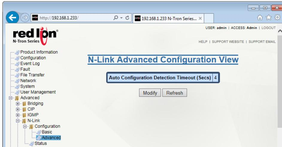
Click on the *Modify* button to change the detection timeout. Click on the *Update* button once the field has been updated with the required information. To save the changes made, return to the *Configuration* menu and click on the *Save* button.
