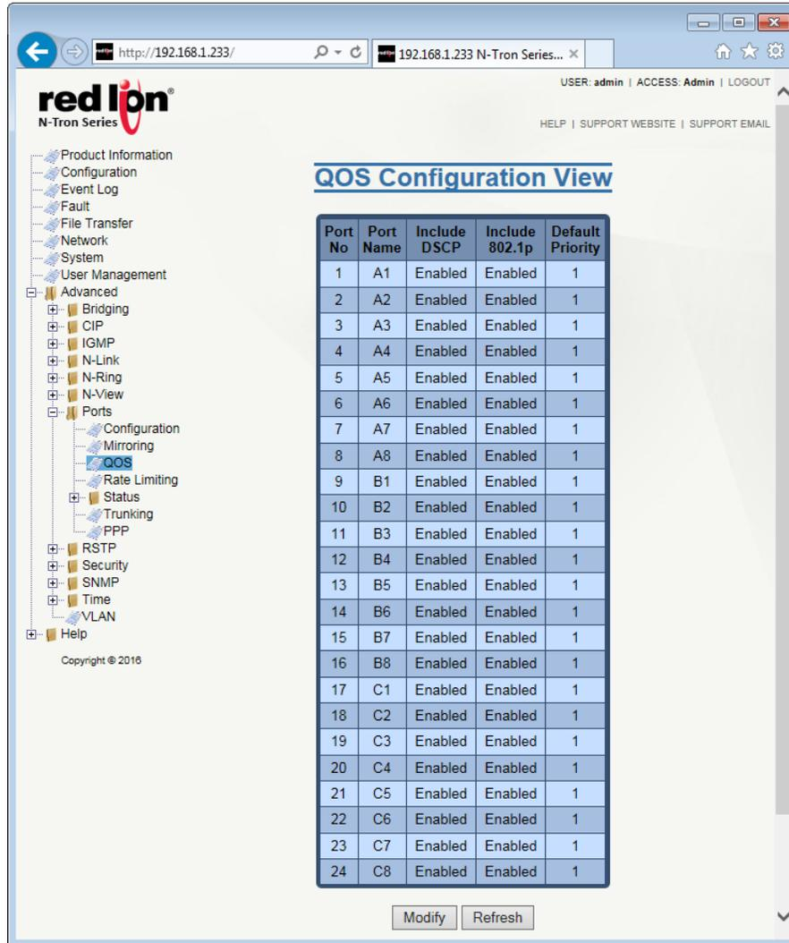
**Include DSCP:** This configurable field displays the status of whether or not to include the ingress frame's RFC 2474 DSCP value in determining the transmit priority and egress frame's IEEE 802.1p User Priority value. If the ingress frame type is IP (IPv4 or IPv6) and Include DSCP is enabled, DSCP processing will override all other settings. (see QOS SELECTION CHART below). The default value is enabled.
