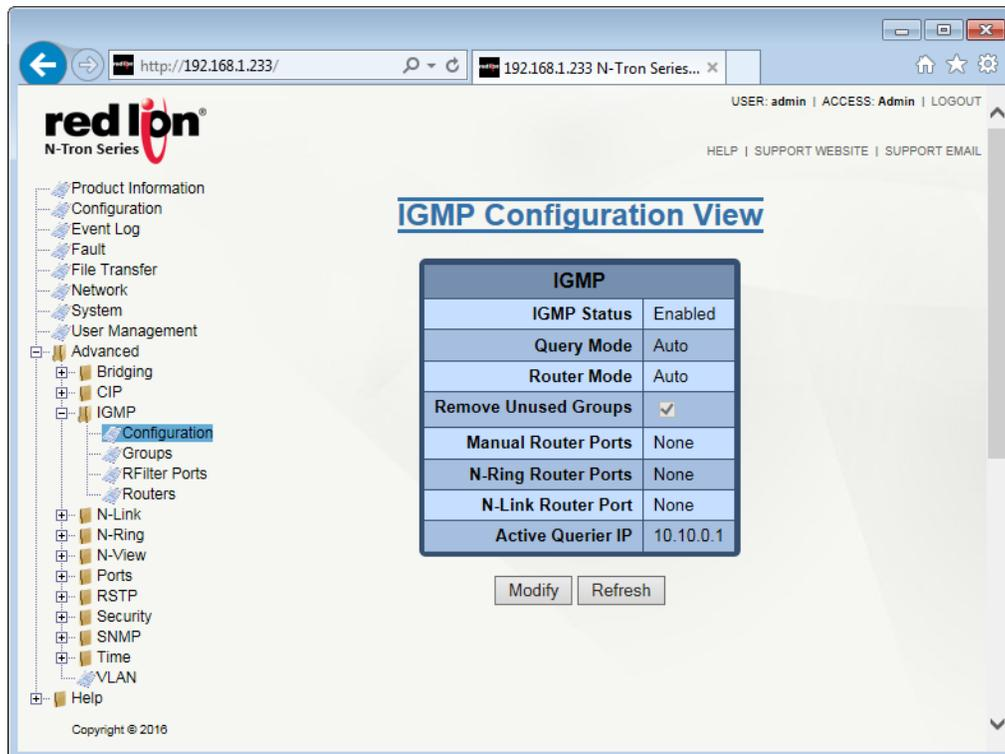
**IGMP Status:** This field indicates whether the IGMP is enabled or disabled. The default value for this field is *Enabled*.
