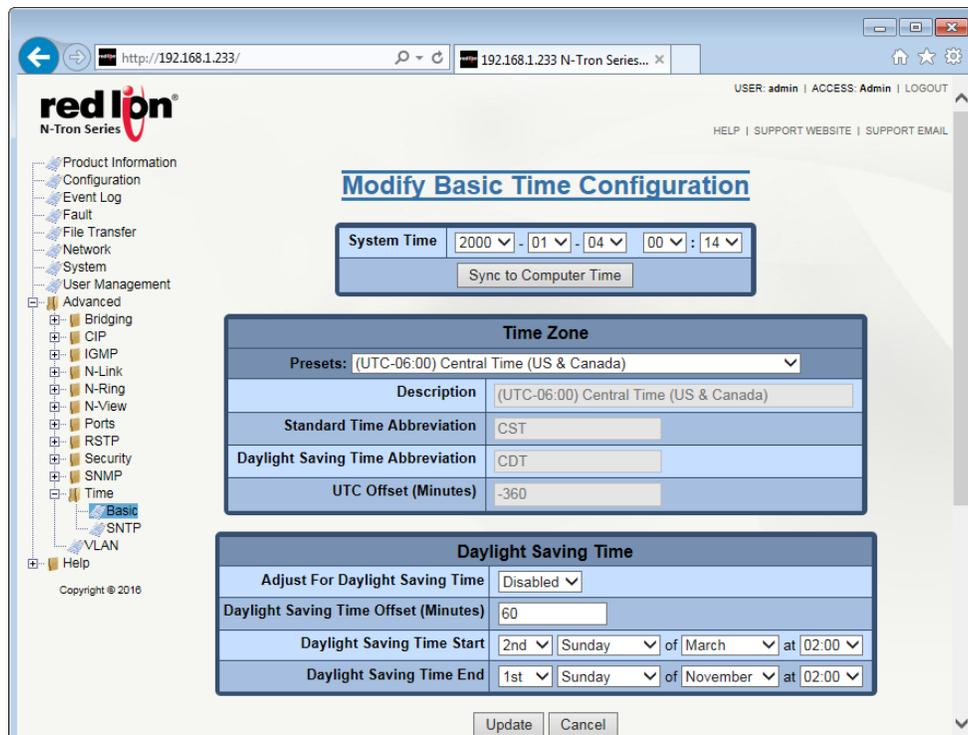
**System Time:** This field displays the date/time of the system. The system date/time defaults to 2000-01-01 00:00:00 CST (UTC-06:00) at system start. The system date/time can be set manually but in the event of a power cycle or reboot it will revert to the default value.
