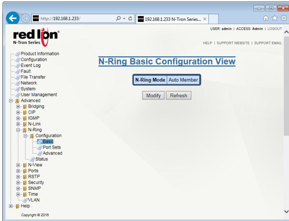
Click on the *Modify* button to make changes to the N-Ring Basic Configuration:
