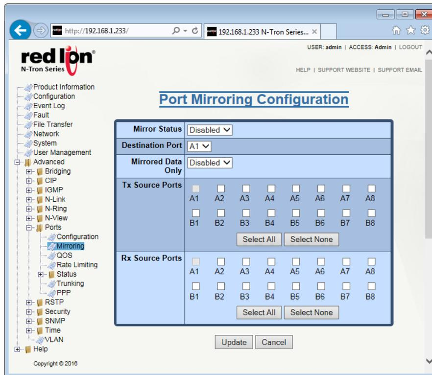
**Mirror Status:** Enable or Disable the Mirroring functionality by selecting the option in the drop-down menu.
