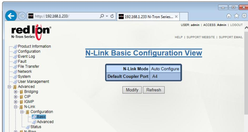
Click on the *Modify* button to make changes. Click on the *Update* button to retain the changes. To save the changes made, return to the Configuration menu and click on the *Save* button.
