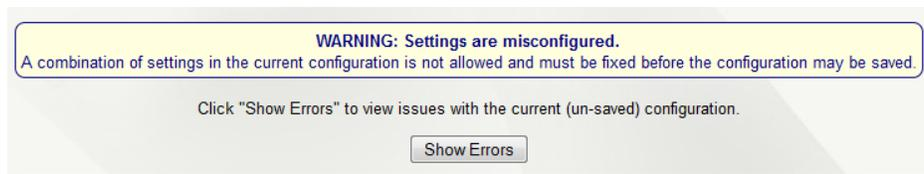
**Show Errors:** Click on the *Show Errors* button to view the current configuration and display any detected errors. This button is only visible when there is a settings misconfiguration.
