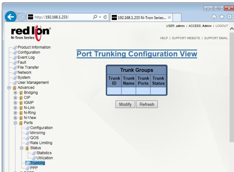
**Trunk ID:** This column displays the trunk identifier number. The valid range is 1-127.
