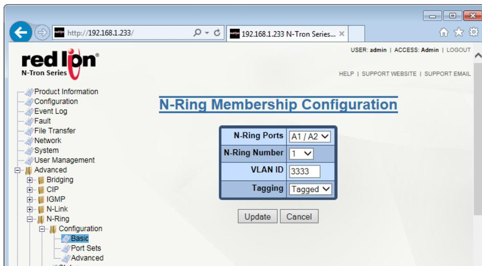
Select the N-Ring Ports and N-Ring Number to be used for the N-Ring. The VLAN ID for each N-Ring Membership must match that of the N-Ring Manager on each specific N-Ring to which the N-Ring Multi-Member will be connected.
