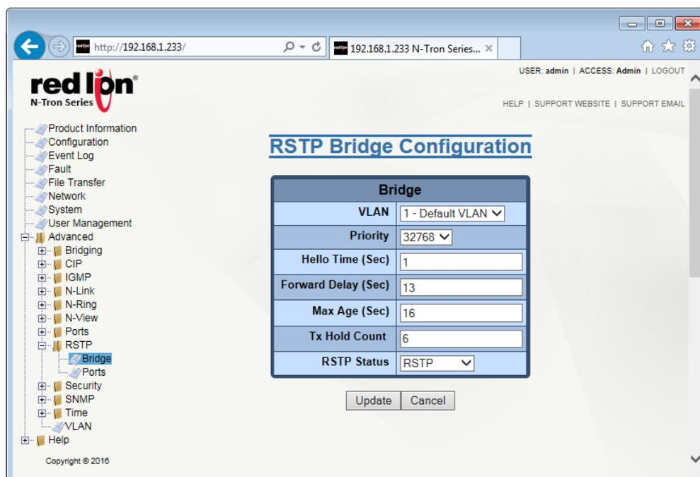
Make the required modifications, and click on the *Update* button. To save the changes made, navigate to the *Configuration* menu and click on the *Save* button.
