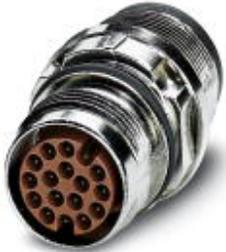
Device connector, front mounting, straight, SPEEDCON locking, M17, Number of positions: 8, Type of contact: Male connector, Crimp connection, Axial O-ring, Central fixing, shielded: yes
