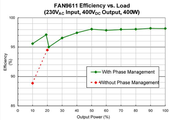
**Figure 63. Measured Efficiency at 230V<sub>AC</sub> (Default Thresholds)**
