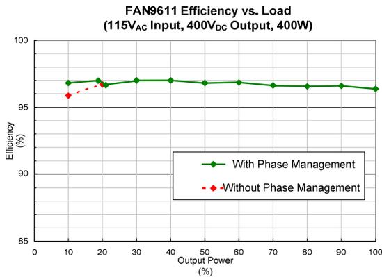
**Figure 62. Measured Efficiency at 115V<sub>AC</sub> (Default Thresholds)**
