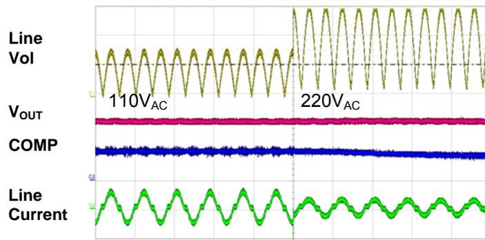
Figure 61. Input Voltage Feedforward
