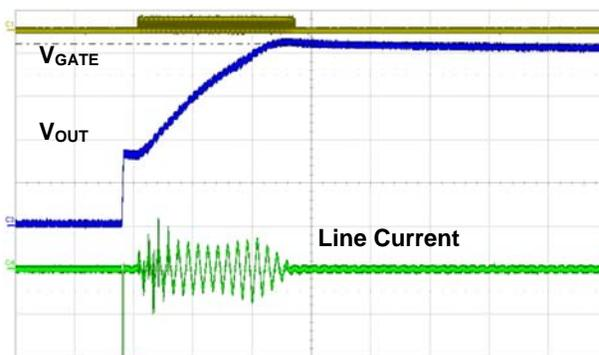
Figure 59. No-Load Startup at 115 V<sub>AC</sub>
