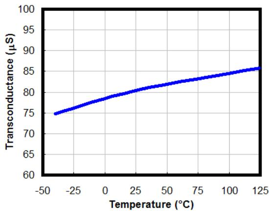
Figure 42. EA Transconductance ( $g_M$ ) vs. Temperature
