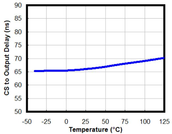
Figure 50. CS to OUT Delay vs. Temperature
