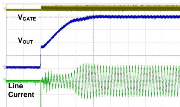
Figure 60. Full-Load Startup at 115 V<sub>AC</sub>
