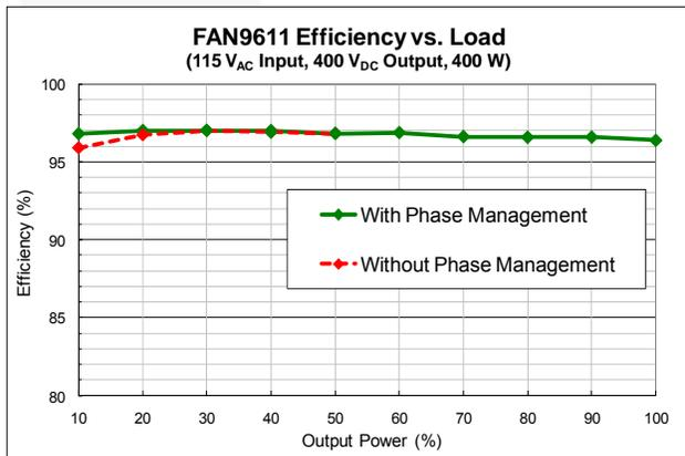
**Figure 64. Measured Efficiency at 115V<sub>AC</sub> (Adjusted Thresholds)**
