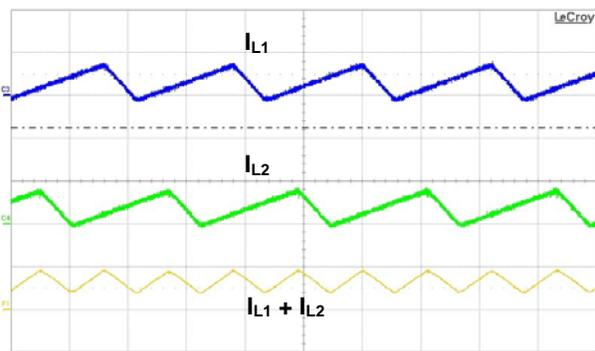
Figure 58. Ripple-Current Cancellation (110 V<sub>AC</sub>)
