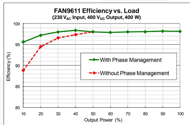
**Figure 65. Measured Efficiency at 230V<sub>AC</sub> (Adjusted Thresholds)**
