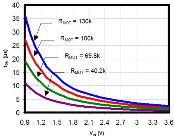
Figure 40. Transfer Function (Maximum On Time vs.  $V_{IN}$ )
