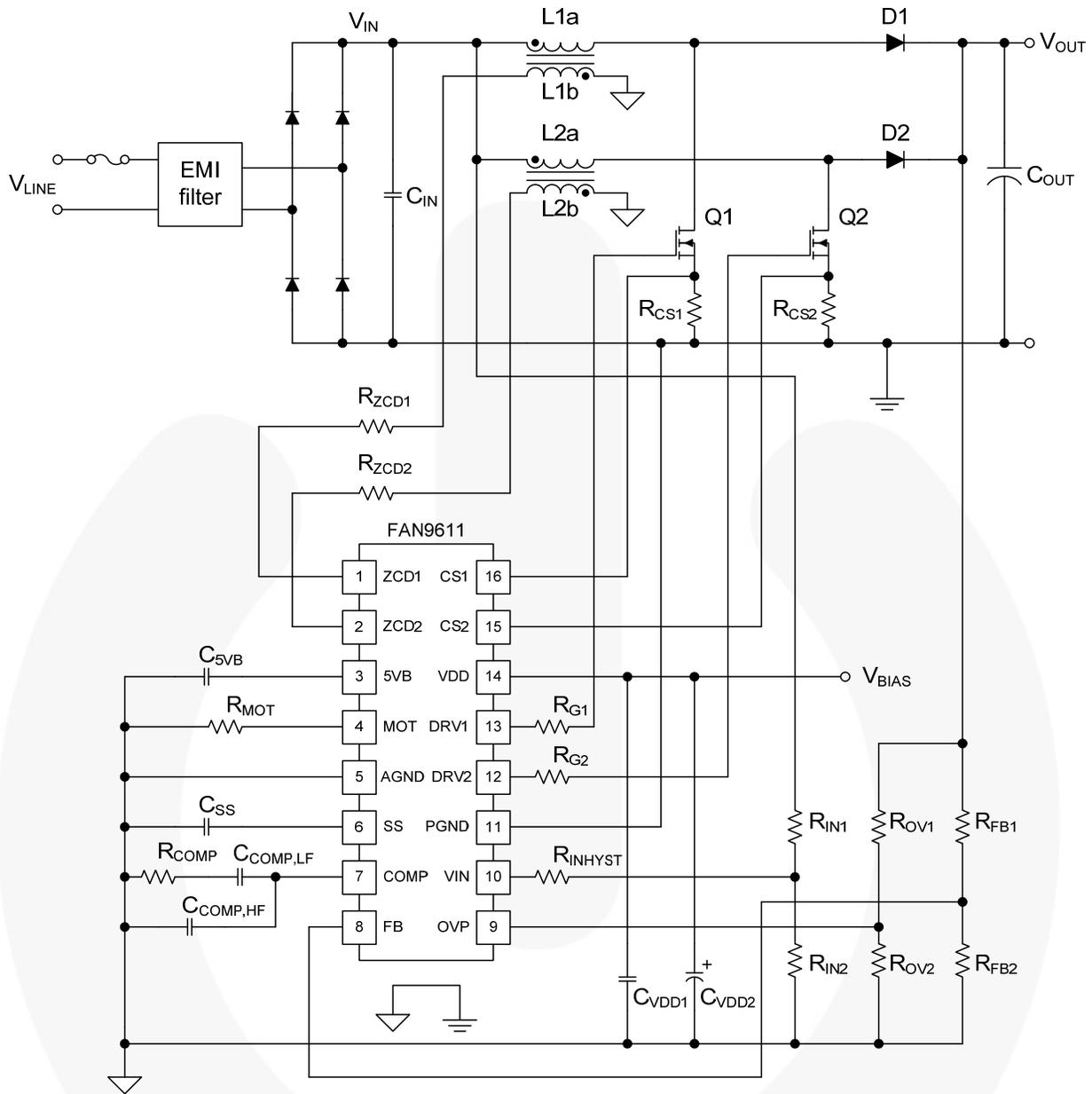
Figure 32. Interleaved BCM PFC Schematic Using FAN9611
