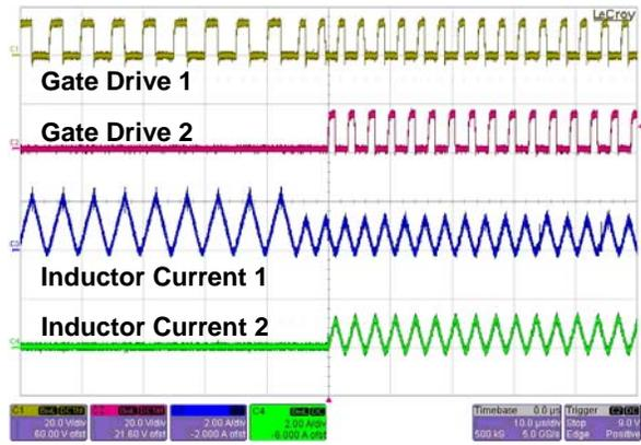
Figure 48. Phase-Adding Operation
