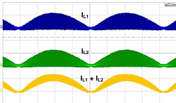
Figure 57. Ripple-Current Cancellation (110 V<sub>AC</sub>)
