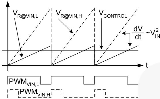
**Figure 10. Input-Voltage Feedforward**
