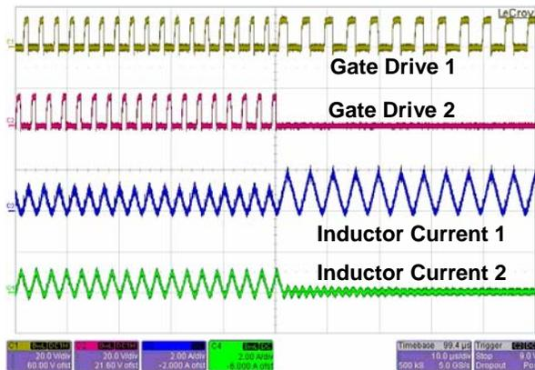
Figure 47. Phase-Dropping Operation
