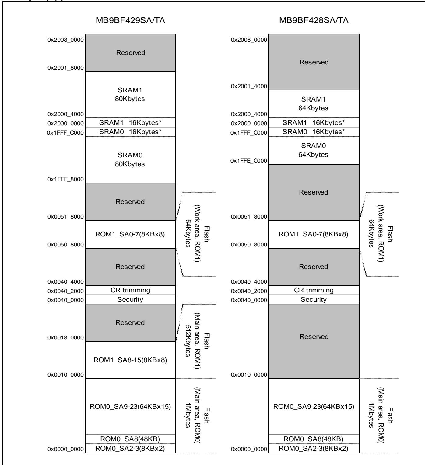
\*: The content of SRAM can be retained at the deep standby modes by the setting of Deep Standby RAM Retention Register (DSRAMR).
