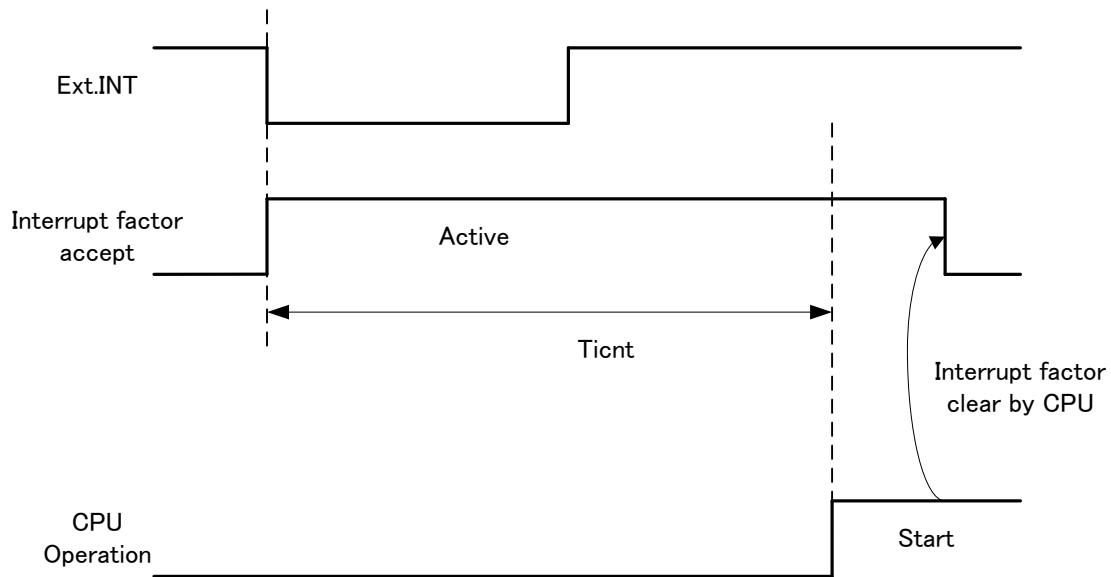
\* : External interrupt is set to detecting fall edge.
