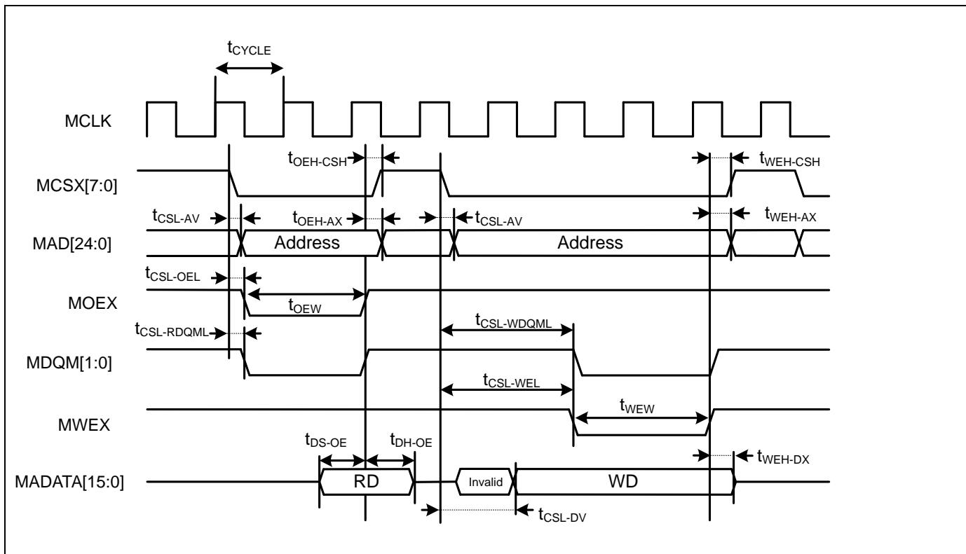
**Separate Bus Access Synchronous SRAM Mode**
