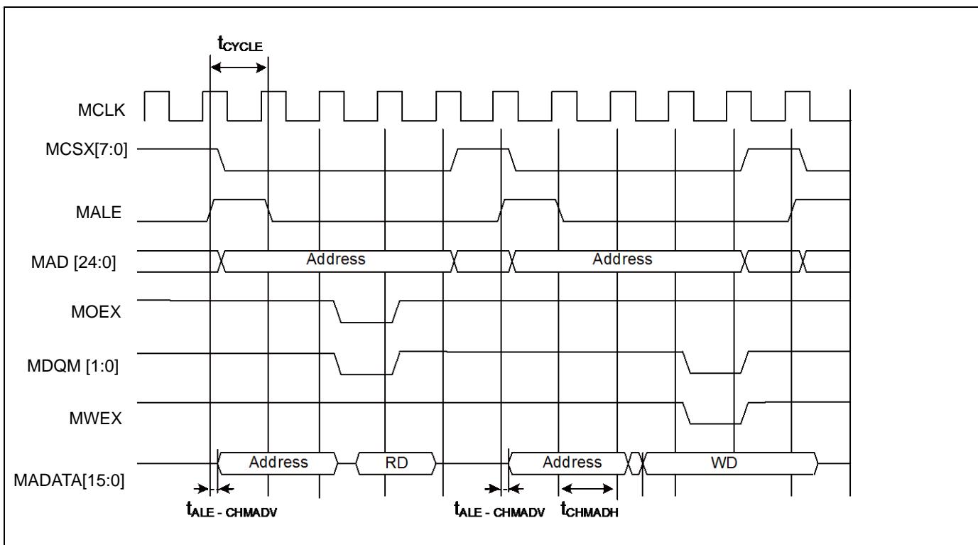
**Multiplexed Bus Access Synchronous SRAM Mode**
