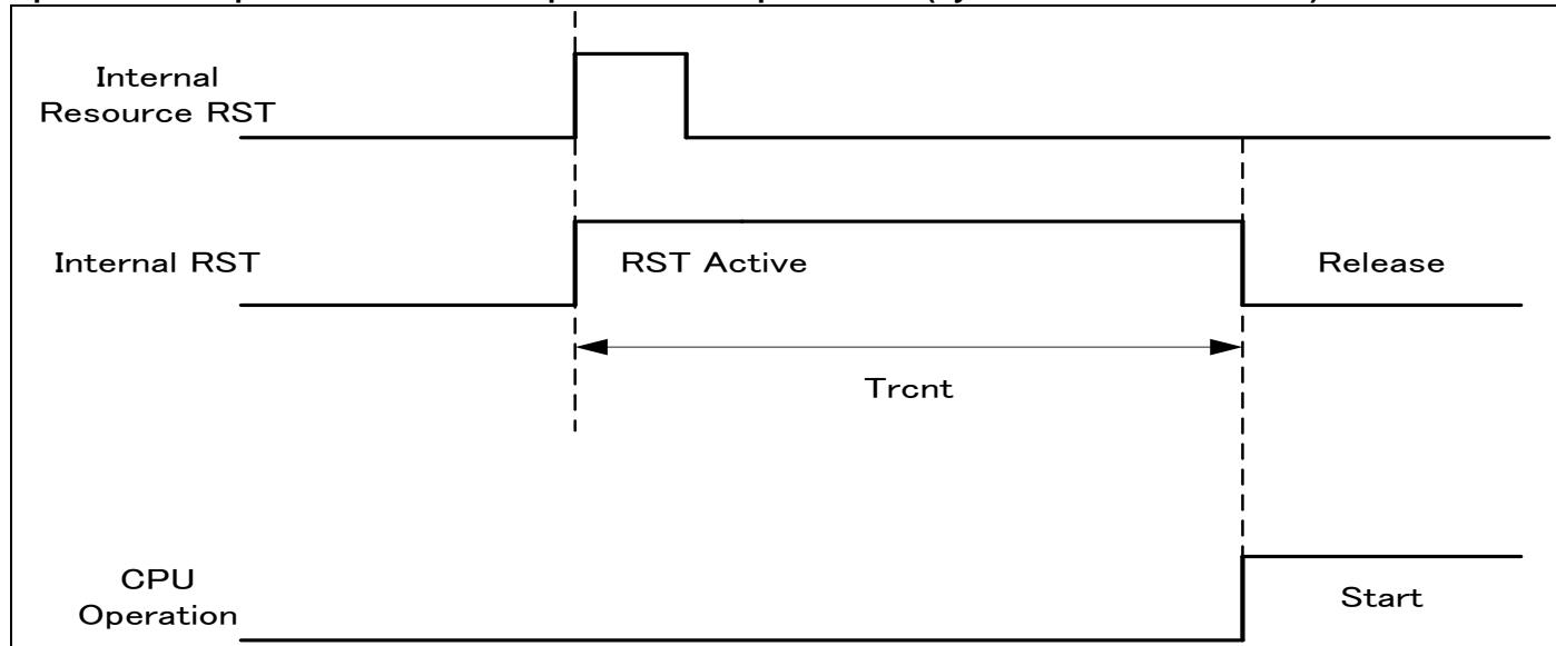
\* : Internal resource reset is not included in return factor by the kind of Low-Power consumption mode.
