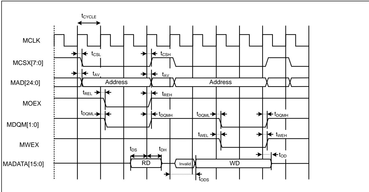
**Multiplexed Bus Access Asynchronous SRAM Mode**
