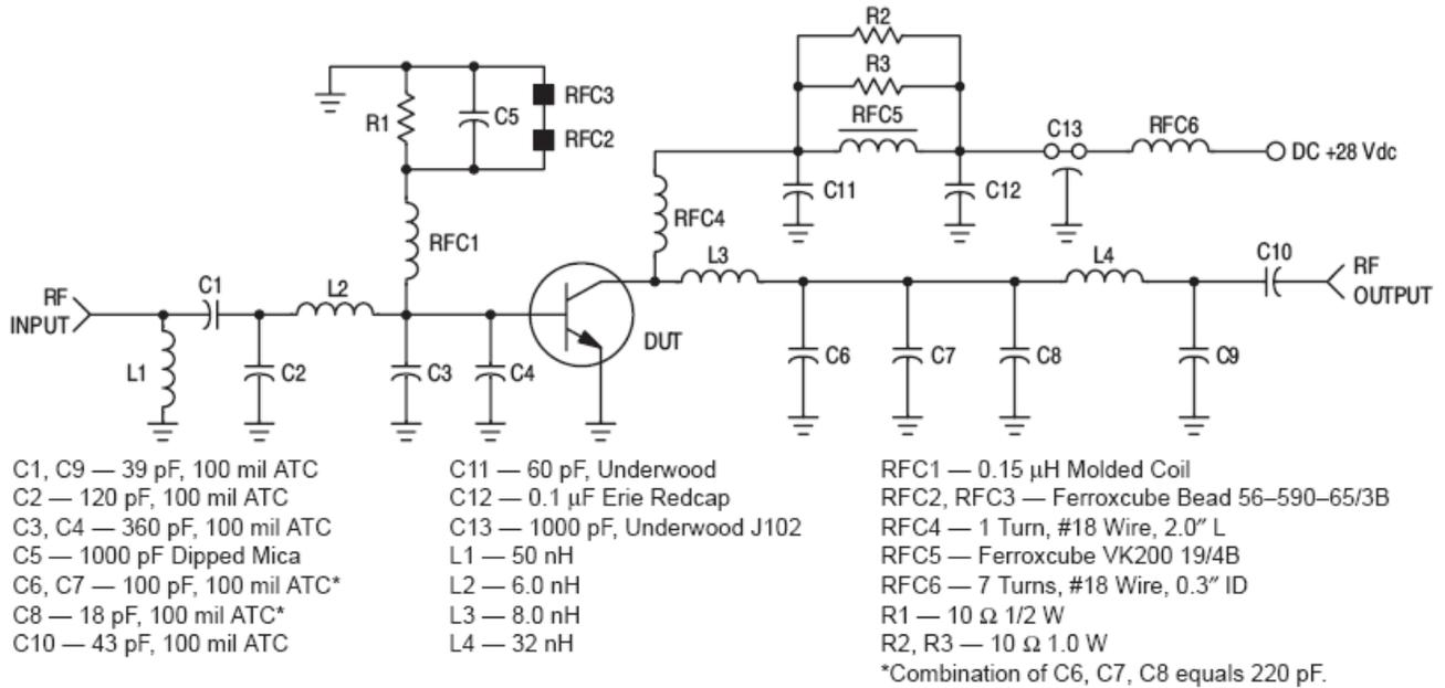
Figure 1. 110–160 MHz Broadband Amplifier — Test Fixture Schematic
