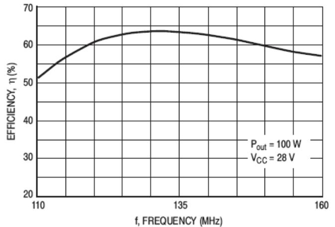
Figure 3. Efficiency versus Frequency
