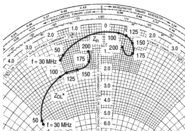
$Z_{OL}^*$  = Conjugate of the optimum load impedance into which the device output operates at a given output power, voltage and frequency.
