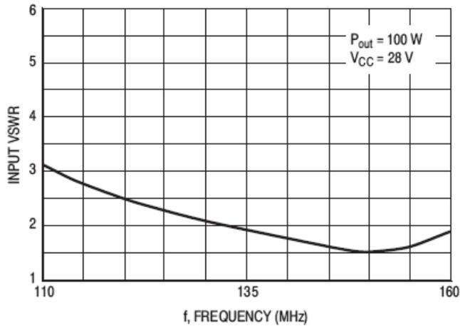
Figure 4. Input VSWR versus Frequency
