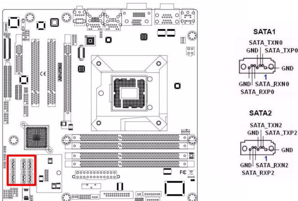
AIMB-581 features a high performance Serial ATA interface (up to 300 MB/s) and Serial ATA III interface (up to 600 MB/s) which eases hard drive cabling with thin, space-saving cables.
