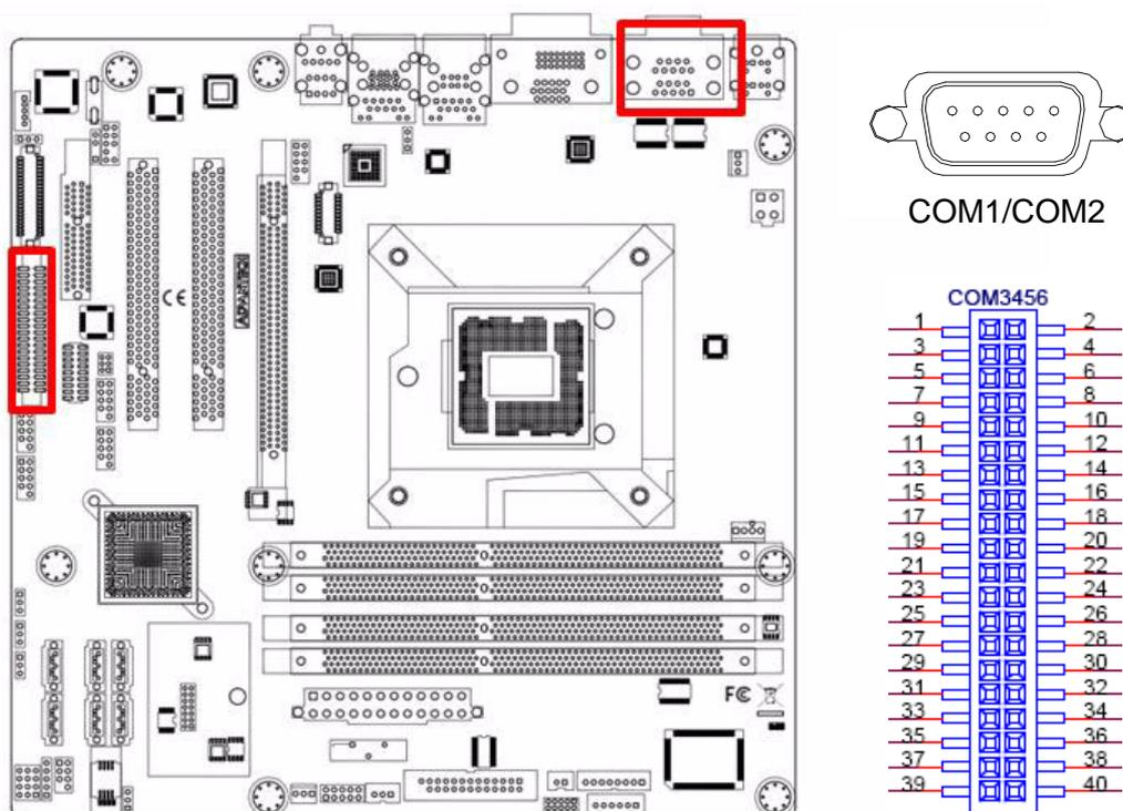
AIMB-581 supports six serial ports. COM1, COM2, COM4-6 supports RS-232. COM3 supports RS-232/422/485(with 5V/12V power). JSETCOM3 is used to select the RS-232/422/485 mode for COM3.
