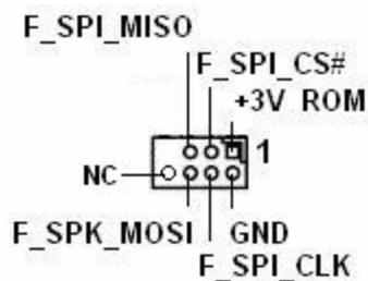
**Table B.4: SPI\_CN1:SPI Fresh Card Pin Connector**
