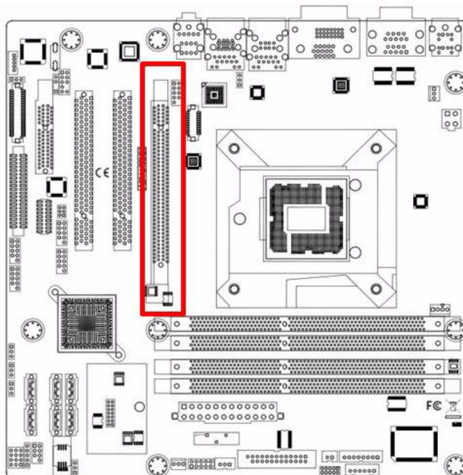
AIMB-581 provides a PCIe x 16 slot for users to install add-on cards when their applications require higher graphic performance than the CPU embedded graphics controller can provide.
