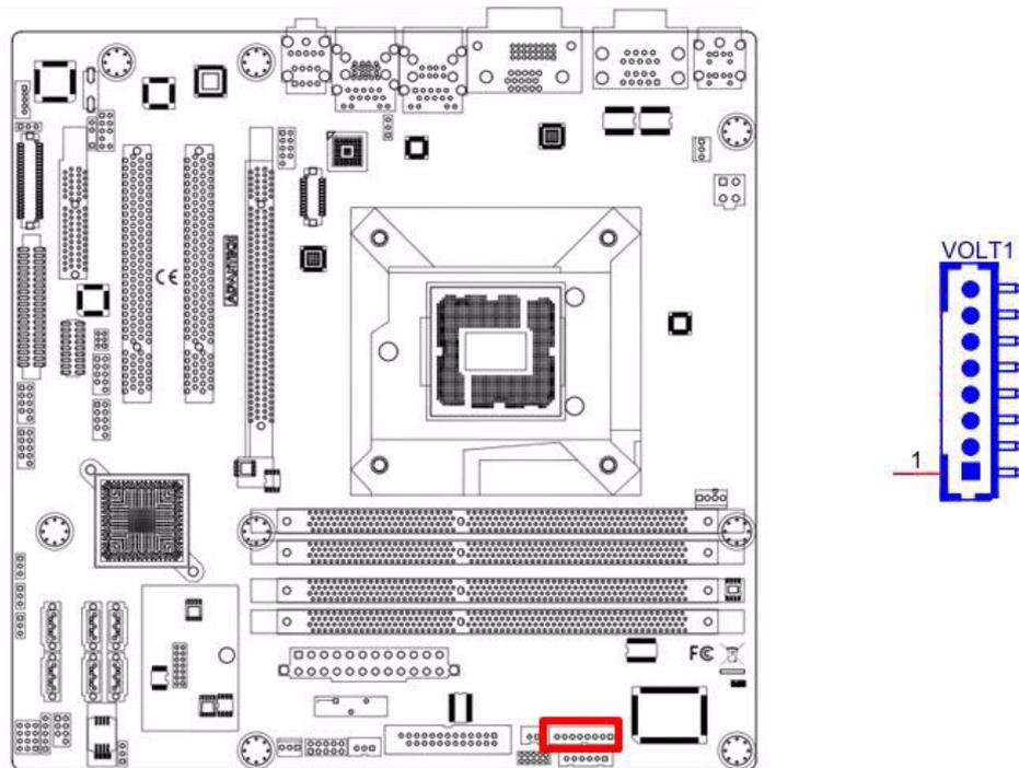
VOLT1 connects to the alarm board of Advantech chassis. These alarm boards give warnings if a power supply or fan fails, if the chassis overheats.
