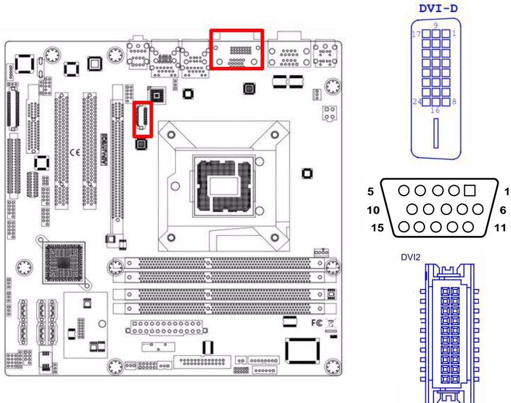
AIMB-581 includes VGA and DVI interface that can drive conventional VGA and DVI displays. VGA is a standard 15-pin D-SUB connector commonly used for VGA. Pin assignment for VGA and DVI connector are detailed in Appendix B.
