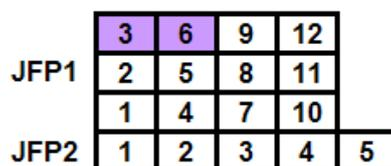
**Table B.10: Power Switch/HDD LED/SMBus/Speaker (JFP1)**
