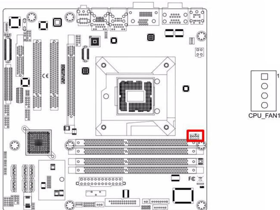
If a fan is used, this connector supports cooling fans of 500 mA (6 W) or less.
