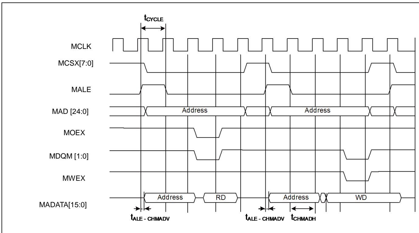
**Multiplexed Bus Access Synchronous SRAM Mode**
