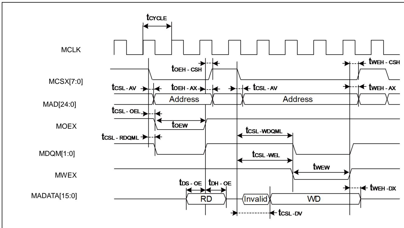
**Separate Bus Access Synchronous SRAM Mode**
