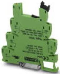
6.2 mm PLC basic terminal block for input functions with screw connection, without relay or solid-state relay, for mounting on DIN rail NS 35/7,5, with sensor supply voltage distribution (BB), 1 N/O contact, input voltage 24 V DC
