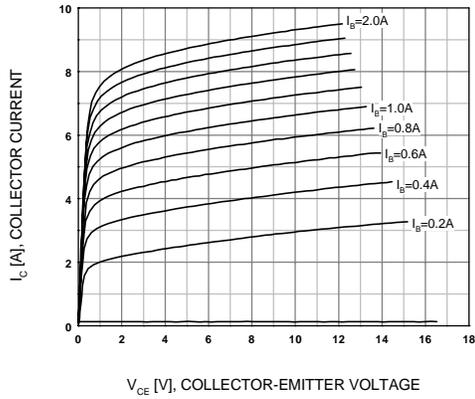
Figure 1. Static Characteristic
