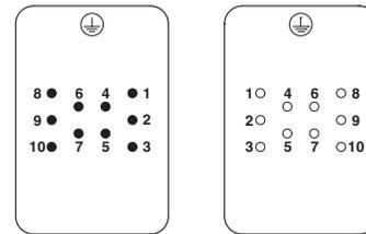
Connector pin assignment: Left pin - right socket
