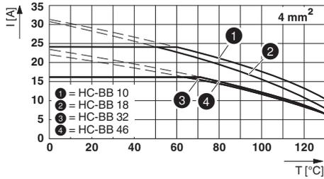
Derating diagram (conductor cross section: 4.0 mm<sup>2</sup>)
