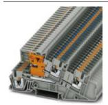
Installation level terminal block, Push-in connection, Cross section: 0.14 mm² - 4 mm², AWG: 26 - 12, Width: 5.2 mm, Color: gray, Mounting type: NS 35/7,5, NS 35/15
