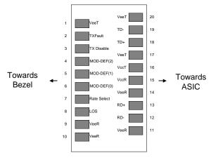
**Pinout of Connector Block on Host Board**
