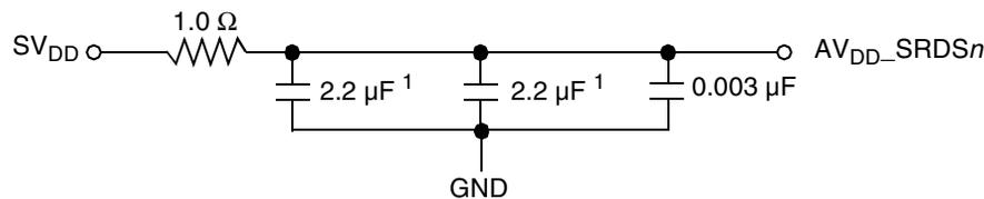
1. An 0805 sized capacitor is recommended for system initial bring-up.
