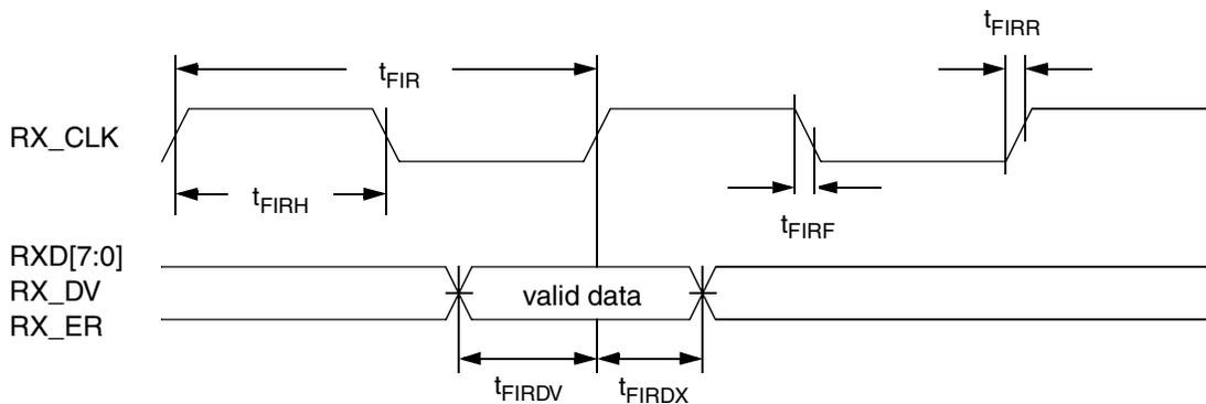
Figure 9. FIFO Receive AC Timing Diagram
