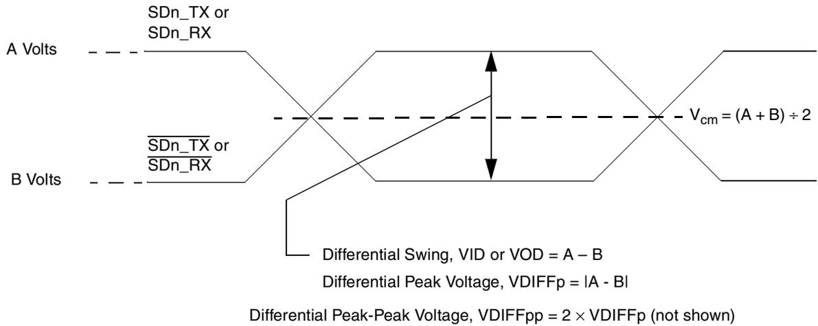
**Figure 38. Differential Voltage Definitions for Transmitter or Receiver**
