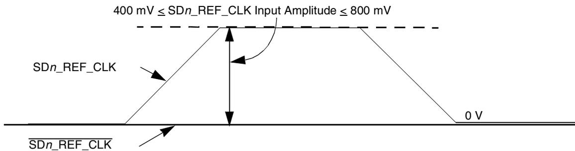
**Figure 42. Single-Ended Reference Clock Input DC Requirements**
