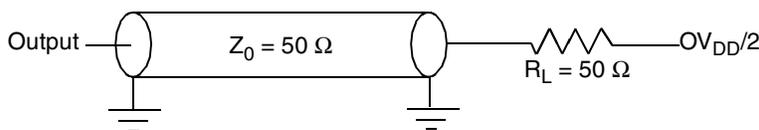
**Figure 36. I<sup>2</sup>C AC Test Load**
