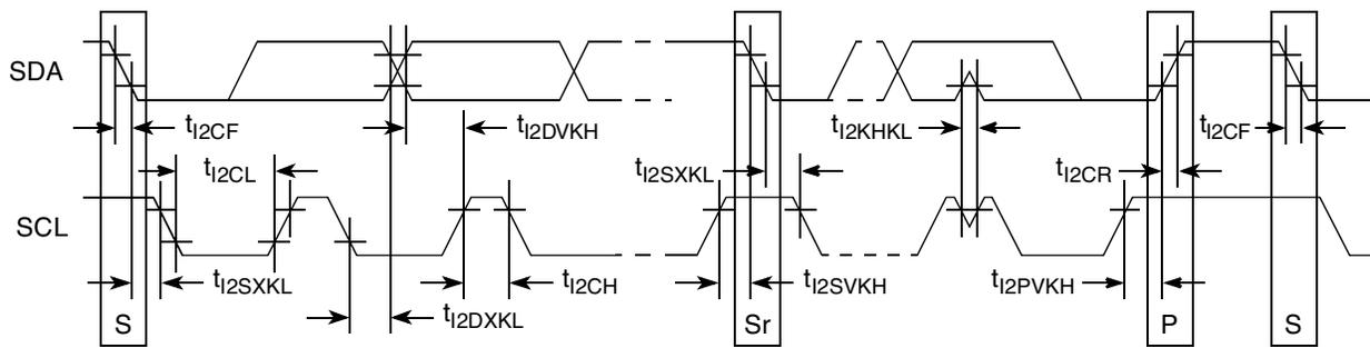
Figure 37. I<sup>2</sup>C Bus AC Timing Diagram
