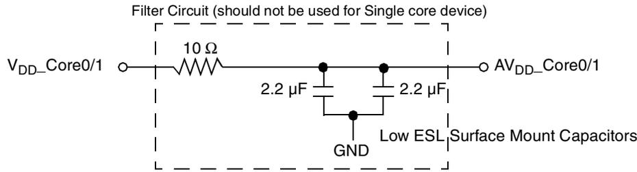
**Note:** For single core device the filter circuit (in the dashed box) should be removed and AV<sub>DD</sub>\_Core1 should be tied to ground with a weak (2–10 kΩ) pull-down resistor.
