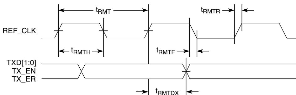
**Figure 20. RMII Transmit AC Timing Diagram****8.2.7.2 RMII Receive AC Timing Specifications**
