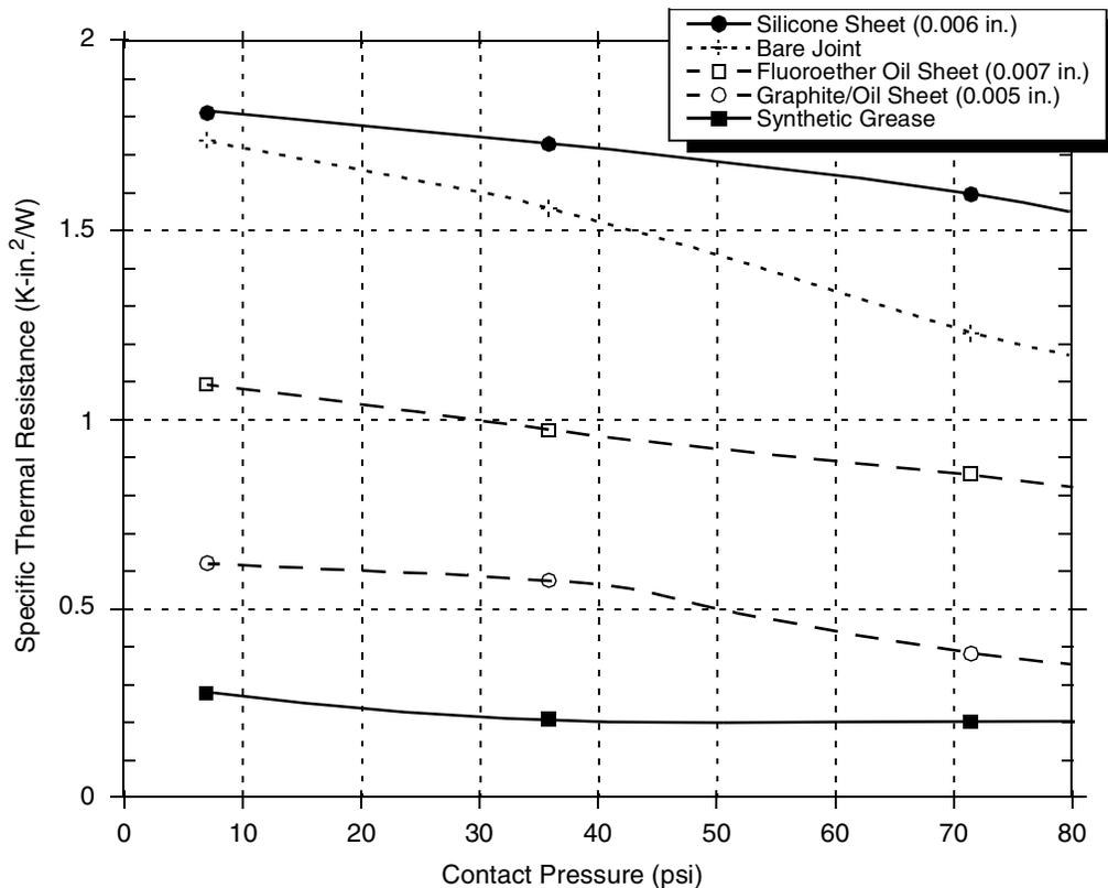
Figure 61. Thermal Performance of Select Thermal Interface Material
