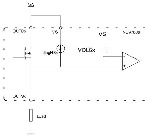
**Figure 29. Open Load Circuitry as High Side Driver**
