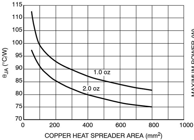
**Figure 35.  $\theta_{JA}$  vs. Copper Heat Spreader**
