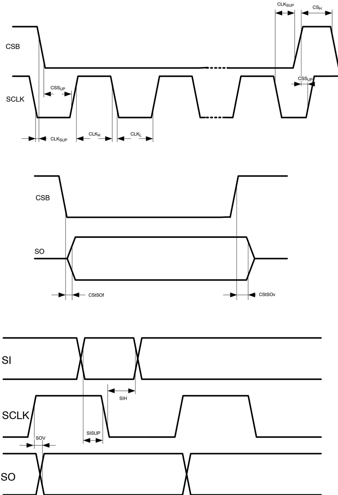
Figure 9. Detailed SPI Timing
