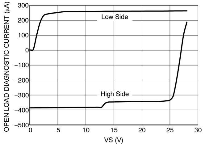
Figure 19. Open Load Detect Current vs. VS @ 25°C
