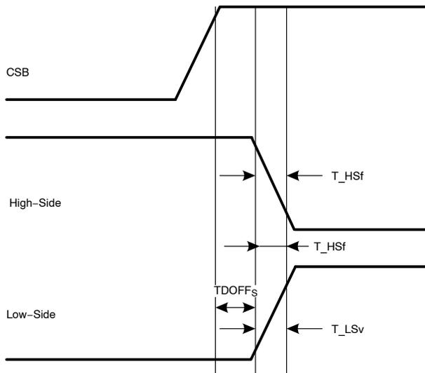
Figure 4. Serial Turn Off
