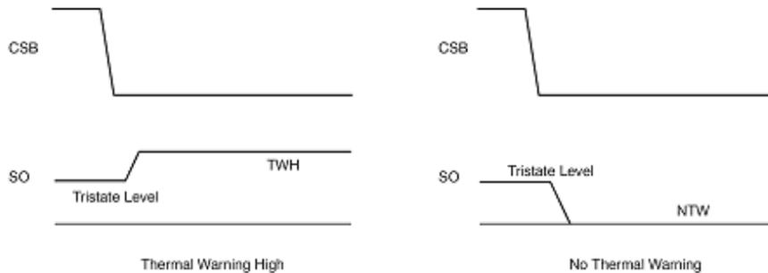
Figure 26. Accessing Thermal Warning Bit
