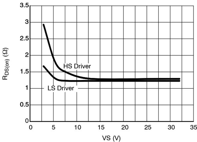
Figure 14. R<sub>DS(on)</sub> vs. VS
