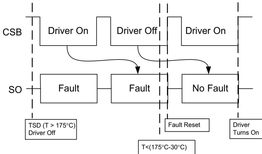
**Figure 33. Thermal Shutdown Timing Diagram**
