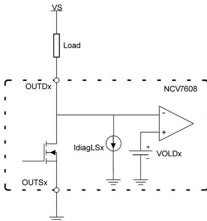
**Figure 28. Open Load Circuitry as Low Side Driver**
