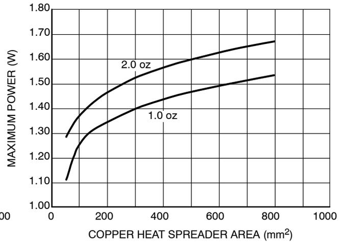
**Figure 36. Maximum Power vs. Copper Heat Spreader**
