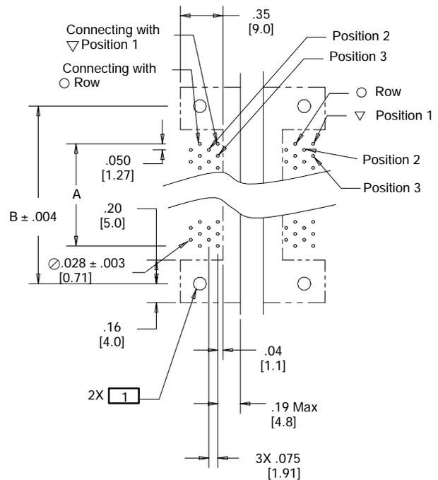
Note: Plated through holes for .062" board thickness
