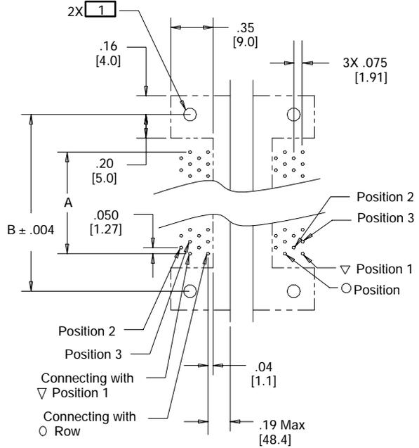
Note: Plated through holes for .062" board thickness
