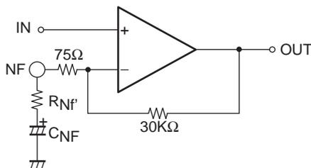
The voltage gain VG can be lowered by connecting an external resistor in series between the NF pin (pins 8 and 14) and CNF.
