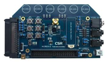
This board features the latest CSR BlueCore® CSR8675 WLCSP Bluetooth audio solution. It interfaces with microphones and has flexible LED and push-button assignments. Battery current measurements can be performed, and a PIO header allows for connection of further application hardware, such as displays.
