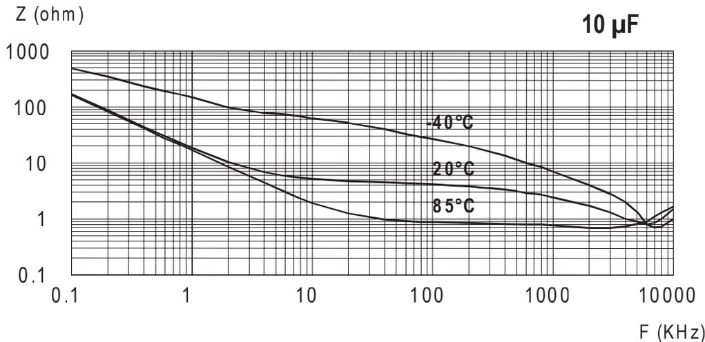
$R_e$  is the most temperature-dependent component of an electrolytic capacitor equivalent circuit. Electrolyte resistivity will decrease if temperature rises.
