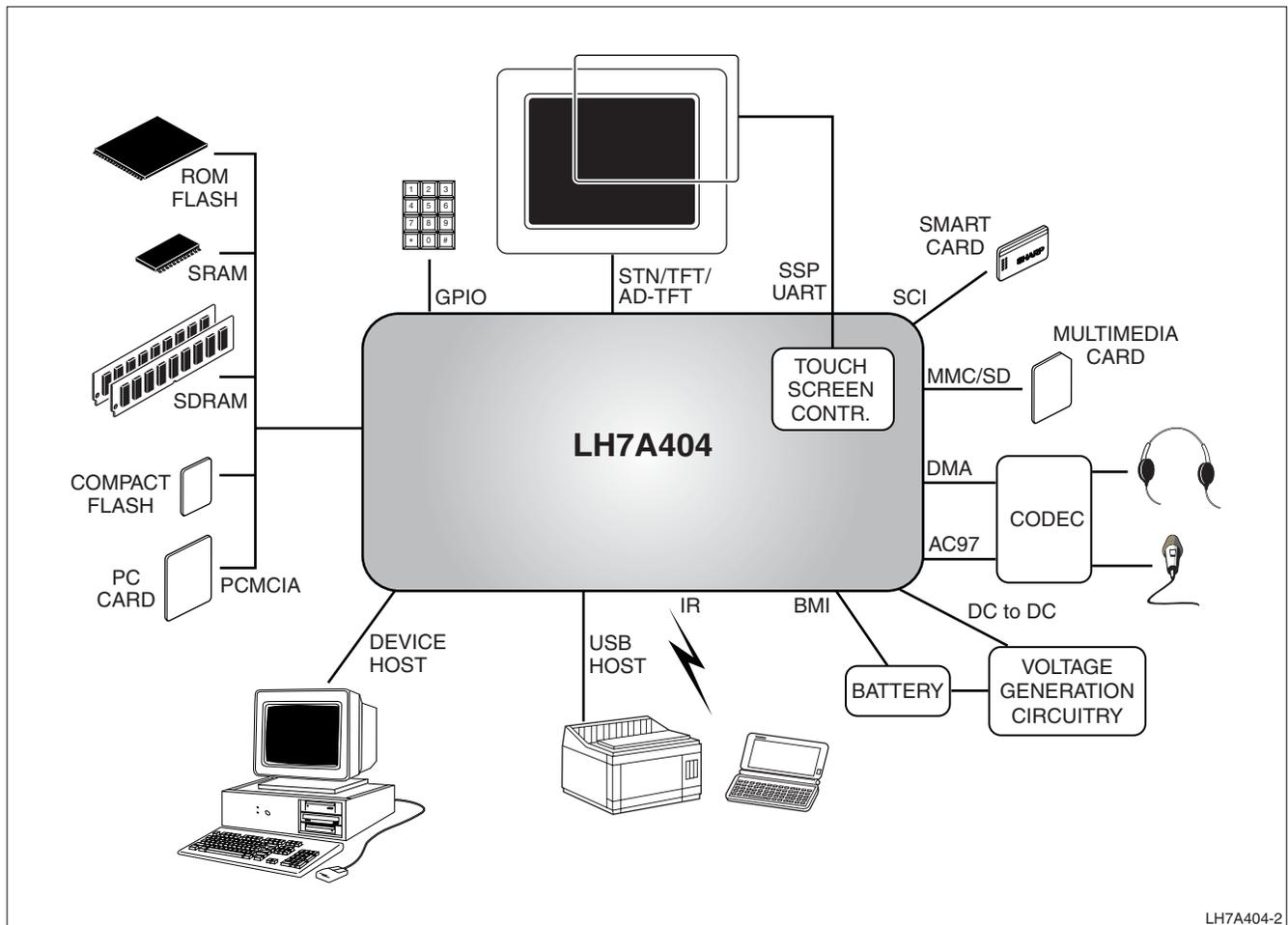
Figure 2. Application Diagram
