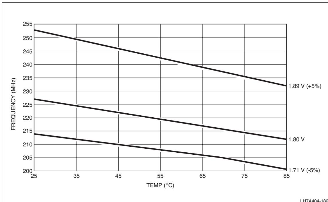
**Figure 5. Temperature/Voltage/Speed Chart (LH7A404-N0E-000-xx and LH7A404-N0F-000-xx Only)**
