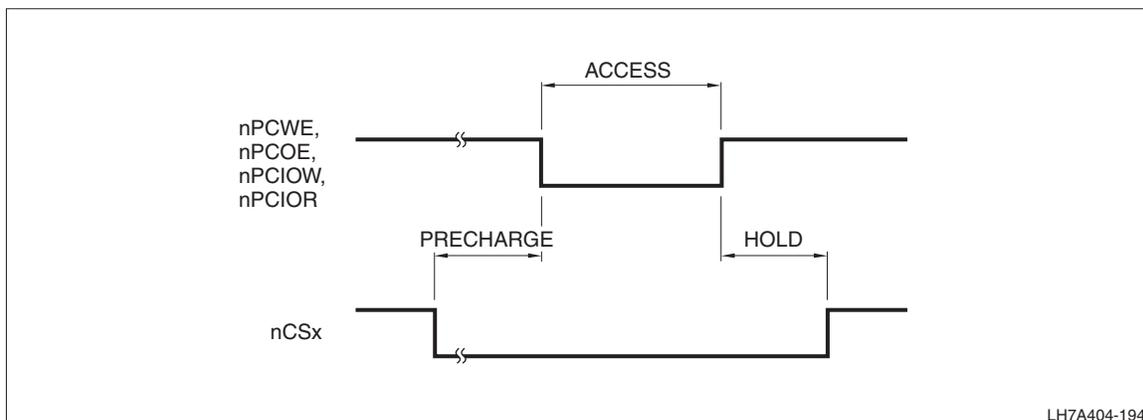
Figure 35. PCMCIA Precharge, Access, and Hold Waveform
