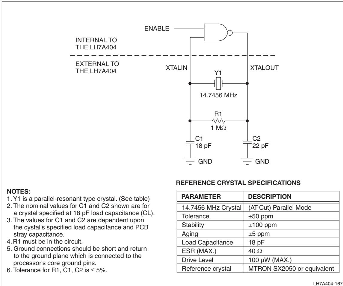
**Figure 53. 14.7456 MHz External Oscillator Components and Schematic**
