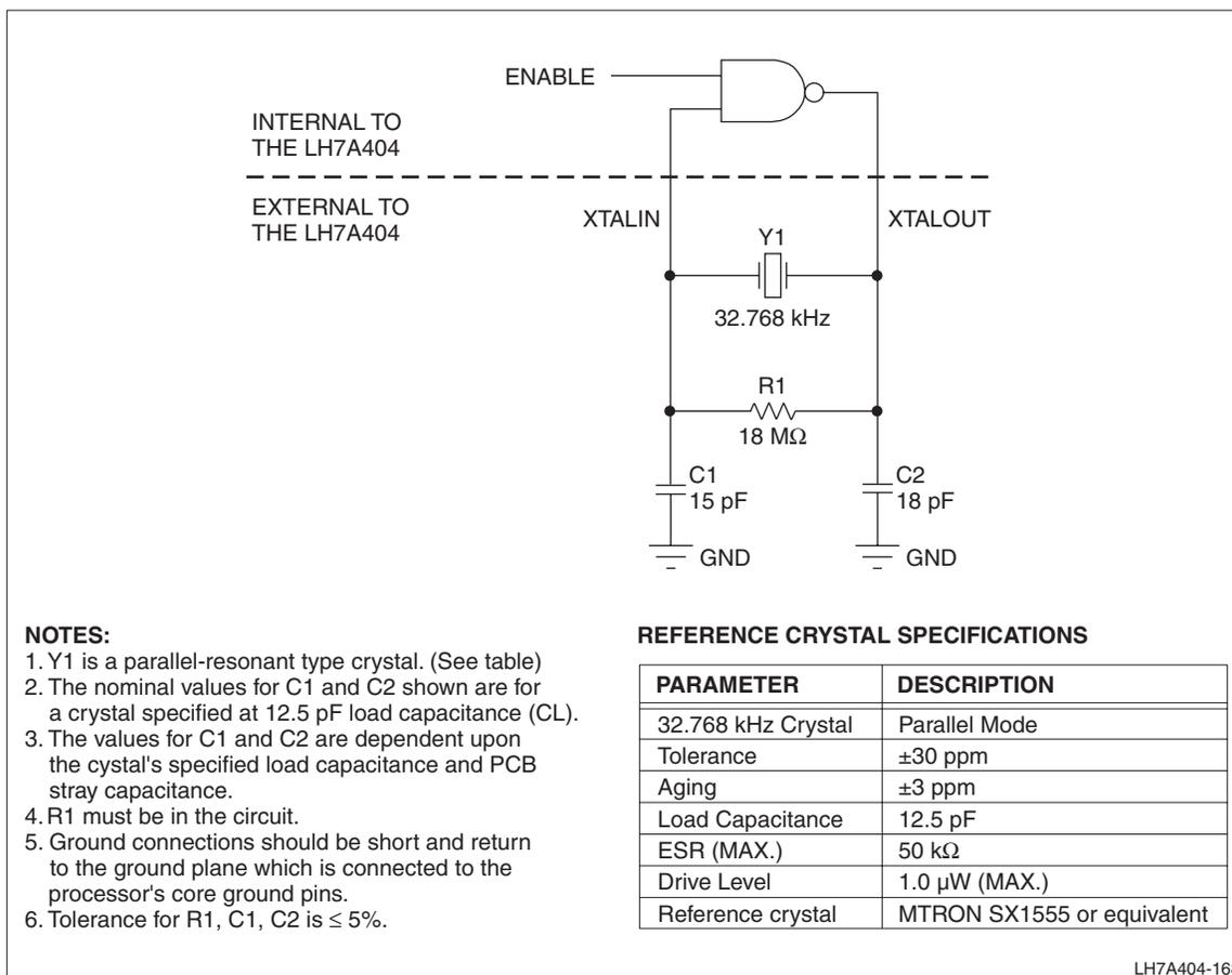
Figure 52. 32.768 kHz External Oscillator Components and Schematic
