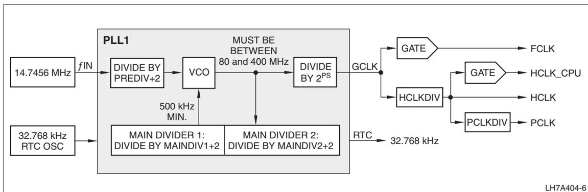
Figure 3. Clock and State Controller Block Diagram
