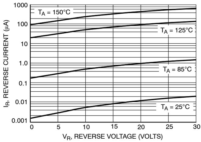
**Figure 3. Leakage Current**
