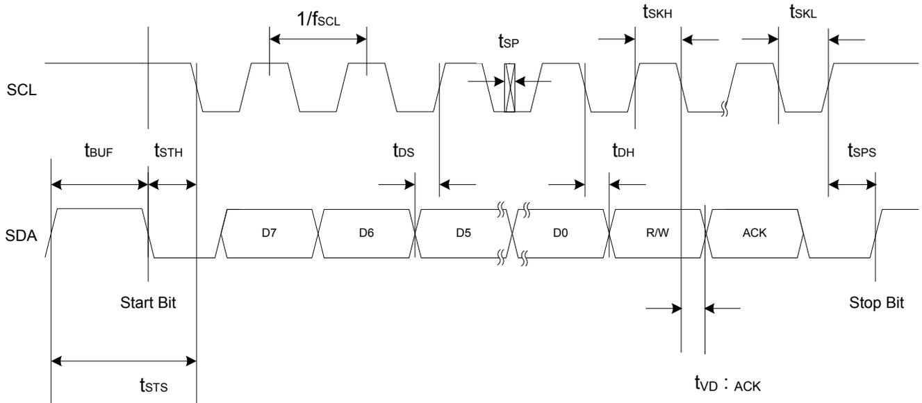
Figure 1. I<sup>2</sup>C Interface Timing Diagram
