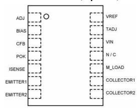
Package 14-Pin DFN with exposed pad 4mm x 3mm 0.50mm pitch 1.5W @T<sub>A</sub>=70°C
