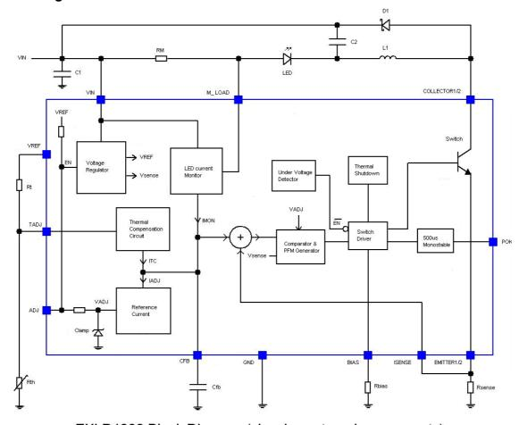
ZXLD1320 Block Diagram (showing external components)
