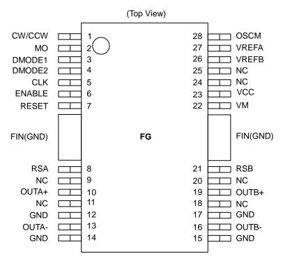
Please mount the FIN of the HSOP package to the GND area of the PCB.
