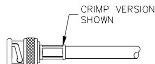
**G** CRIMP OUTER FERRULE WITH APPROPRIATE CRIMP TOOL.
