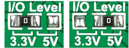
There is one zero-ohm SMD jumper **J1** which is used to select whether 3.3V or 5V I/O voltage level is used. Jumper **J1** is soldered in 3.3V position by default.
