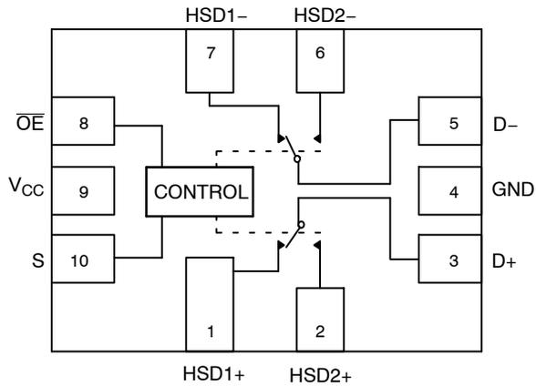
**Figure 1. Pin Connections and Logic Diagram**
