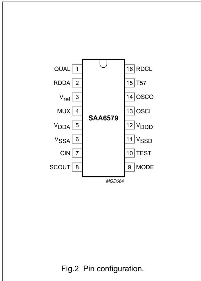
Fig.2 Pin configuration.
