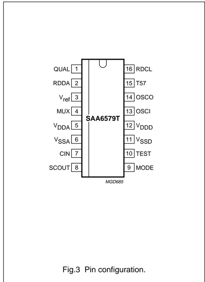
Fig.3 Pin configuration.
