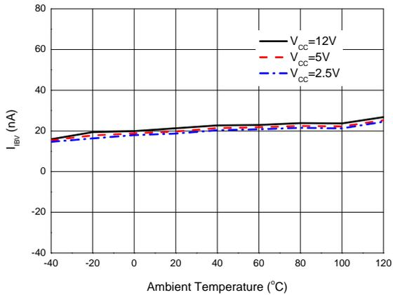
**I<sub>CTRL</sub> Pin Input Bias Current vs. Ambient Temperature**
