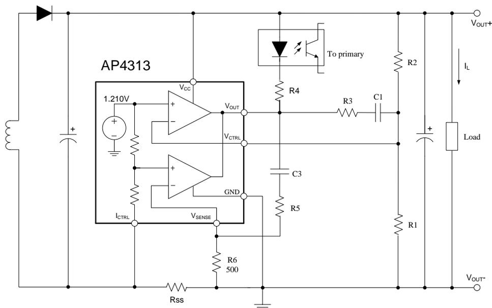
$$V_{OUT} = V_{REF} \times \frac{R1 + R2}{R1} \text{ (V)}$$
