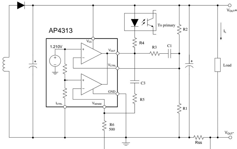
$$V_{OUT} = V_{REF} \times \frac{R1 + R2}{R1} - (I_L \times R_{SS}) \text{ (V)}$$
