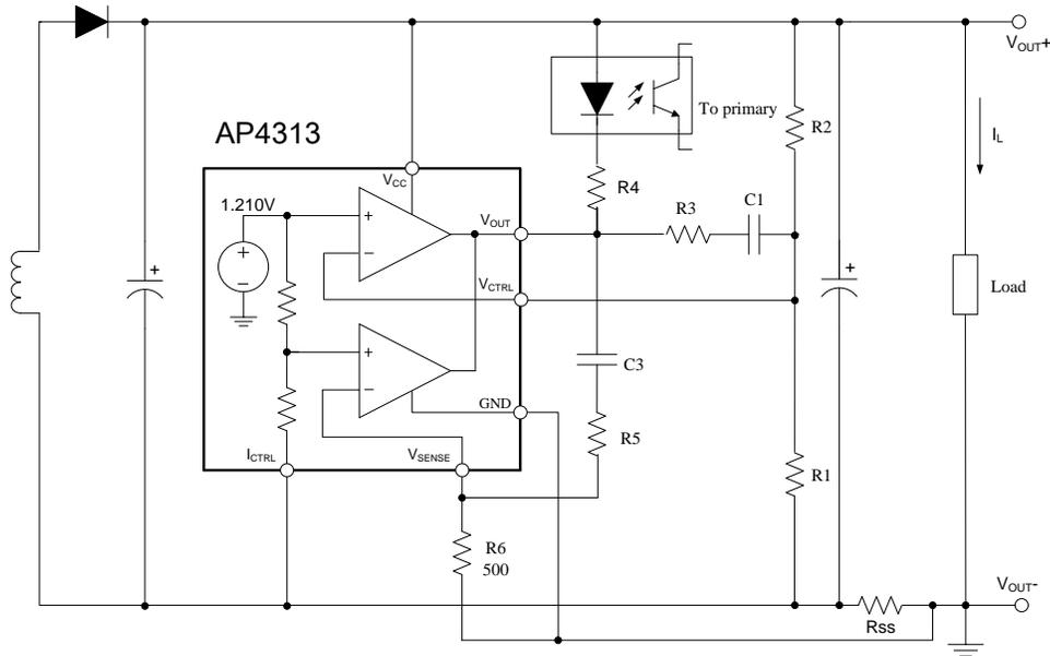
$$V_{OUT} = [V_{REF} + (I_L \times R_{SS})] \times \frac{R1 + R2}{R1} - (I_L \times R_{SS}) \text{ (V)}$$
