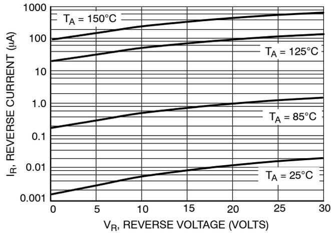
**Figure 3. Leakage Current**
