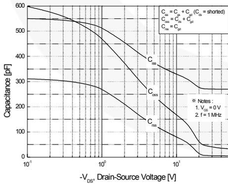
Figure 5. Capacitance Characteristics
