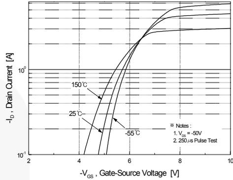
Figure 2. Transfer Characteristics
