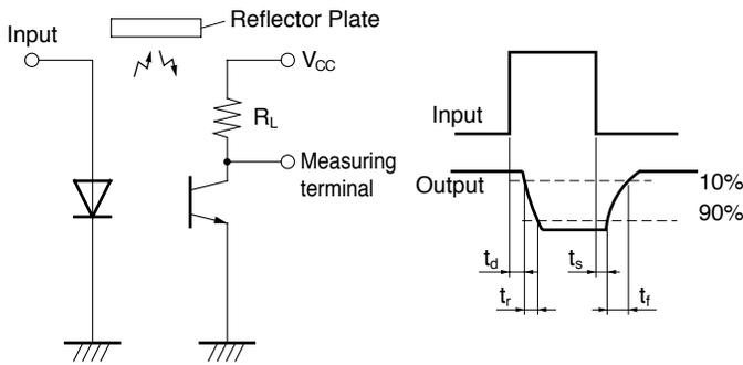
**Fig.10 Detecting Position Characteristics (1)**
