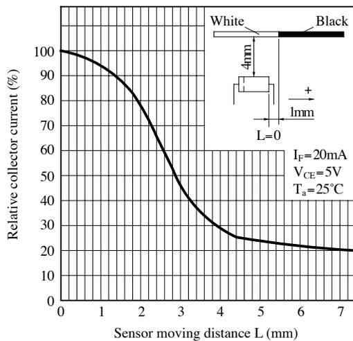
**Fig.12 Relative Collector Current vs. Distance (Reference value)**
