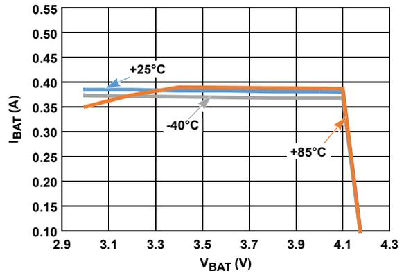
FIGURE 7. CHARGE CURRENT vs OUTPUT VOLTAGE,  $R_{IREF} = 200\text{k}$
