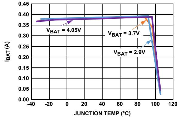
FIGURE 9. CHARGE CURRENT vs JUNCTION TEMPERATURE,  $R_{IREF} = 200\text{k}$
