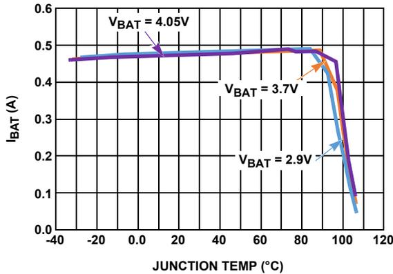
FIGURE 8. CHARGE CURRENT vs JUNCTION TEMPERATURE,  $R_{IREF} = 158\text{k}$
