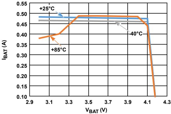
FIGURE 6. CHARGE CURRENT vs OUTPUT VOLTAGE,  $R_{IREF} = 158\text{k}$
