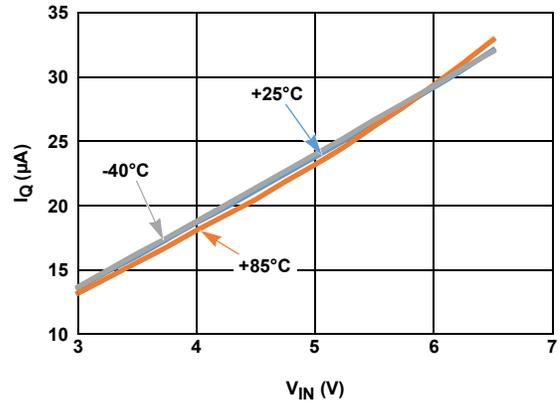
FIGURE 15. INPUT QUIESCENT CURRENT vs INPUT VOLTAGE, SHUTDOWN
