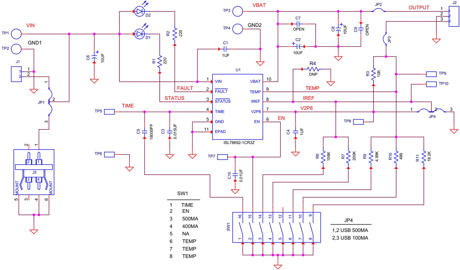
FIGURE 3. ISL78692EVAL1Z SCHEMATIC
