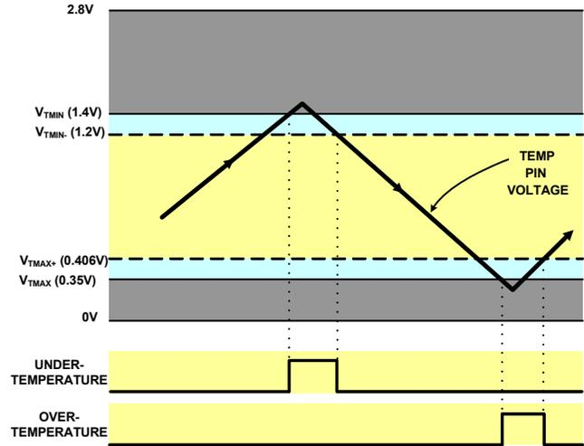
FIGURE 22. CRITICAL VOLTAGE LEVELS FOR TEMP PIN
