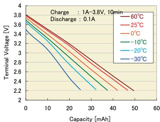
Figure14 Temperature Characteristic of LIC
