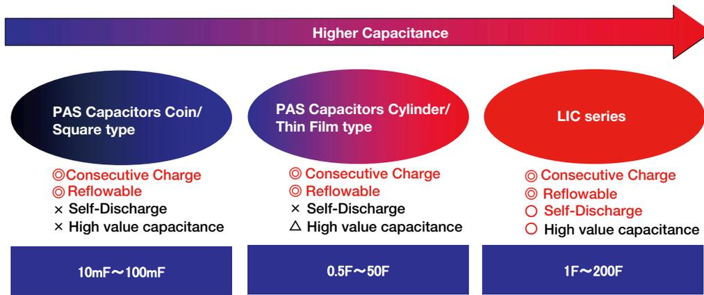
Figure 20 Differences in Usage of PAS Capacitors and LICs
