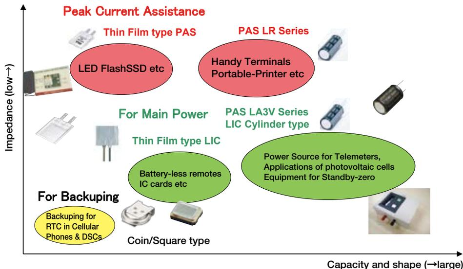
Figure 21 Application of PAS capacitor and LIC
