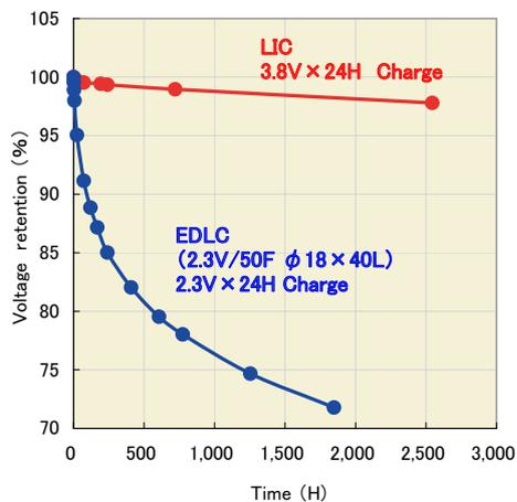
Figure15 Comparison of Self Discharge characteristics Between LIC and Symmetrical EDLC (25°C)
