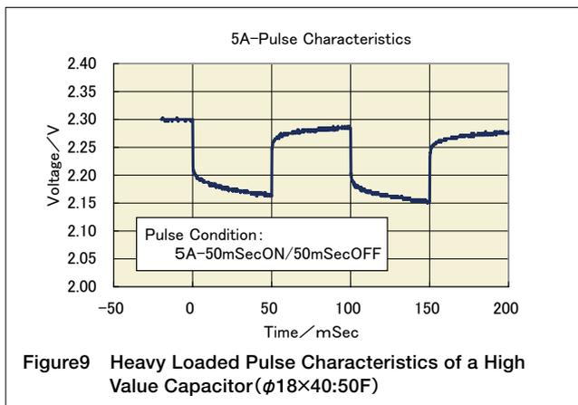
tance with low ESR. As seen by the discharge characteristics and heavy load pulse characteristics in Figures 8 and 9, we offer various types of capacitors for applications that require high capacitance or high power density (for example in handling fluctuations in discharge loads or in charge loads during energy regeneration).
