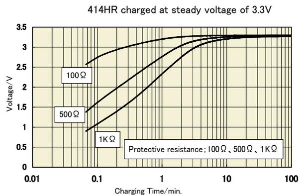
Figure4 Charge Characteristics of PAS414HR
