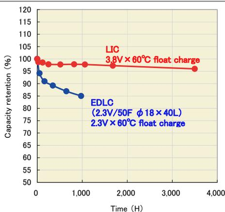
Figure16 High Temperature Loaded Characteristics of LIC and Symmetrical EDLC (Change rate in capacitance at 60°C celsius consecutively charging rated voltage)
