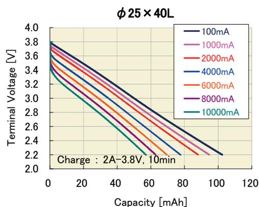
Figure12 Discharge Rate Characteristics of Cylinder type LIC (φ25×40:200F) (25°C)
