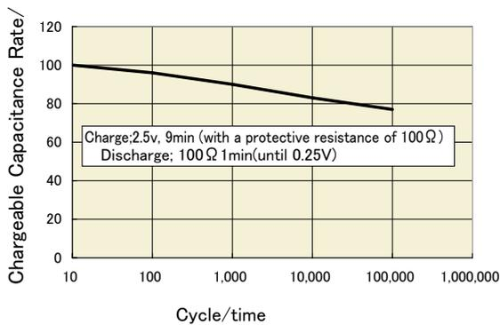
Figure3 Change of Chargeable Capacitance Rate in Cycle
