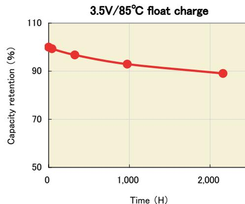
Figure17 High Temperature Loaded Characteristics of LIC (Change rate in capacitance at 85°C-3.5 V consecutive charging)
