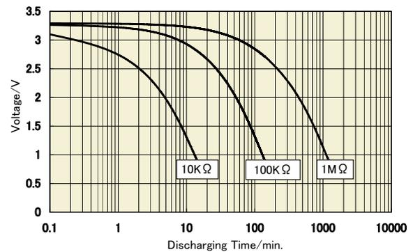
Figure5 Discharge Characteristics of PAS414HR
