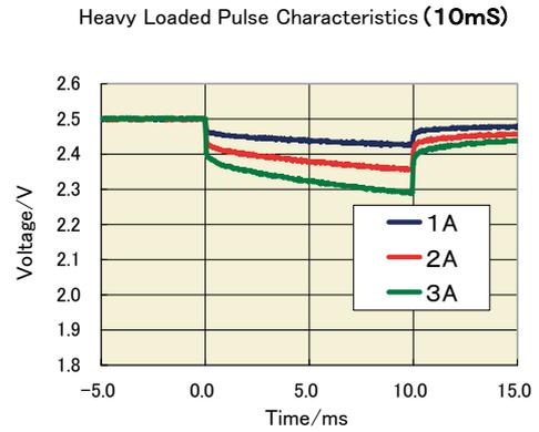
Figure7 Heavy Loaded Pulse Characteristics of a Low ESR-PAS Capacitor ( $\phi 8 \times 15:1F$ )
