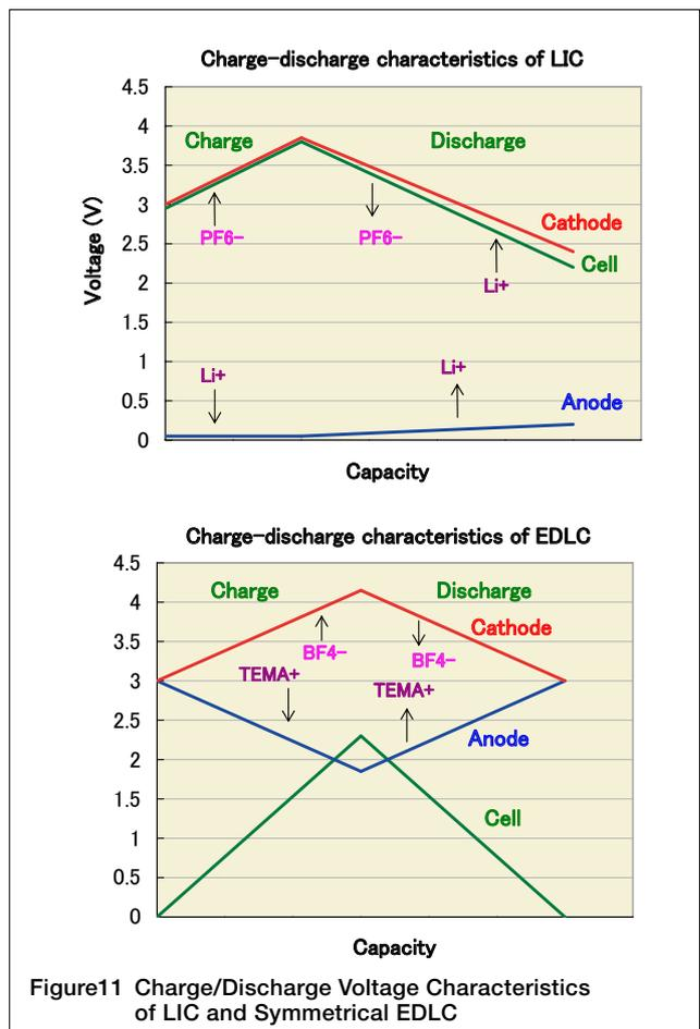
Figure11 Charge/Discharge Voltage Characteristics of LIC and Symmetrical EDLC
