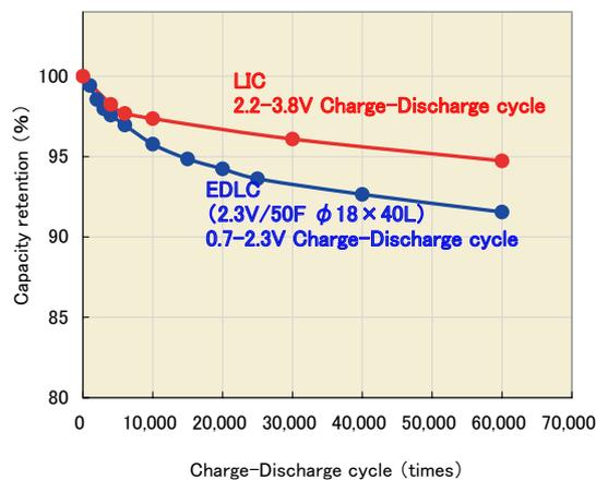
Figure18 Charge-Discharge Cycle characteristics of LIC and symmetrical EDLC
