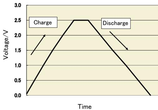
Figure2 Charge/Discharge Curve of a PAS Capacitor
