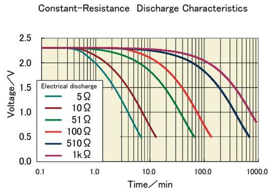
Figure8 Discharge Characteristics of High value Capacitors ( $\phi 18 \times 40:50F$ )
