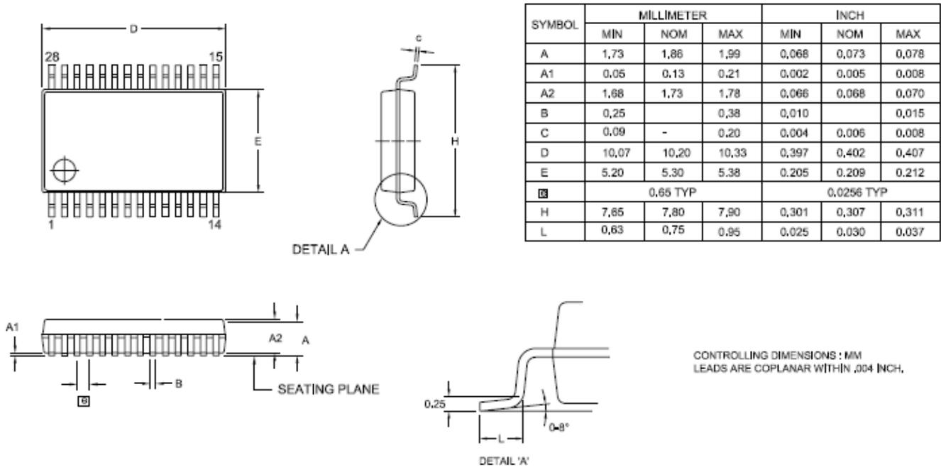
Figure 9 - 28-Pin Small Shrink Outline Package (SSOP)
