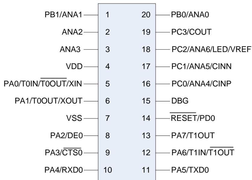
**Figure 3 – 20 Pin SSOP Package Pin-Out – Z8FS040xHH20EG**
