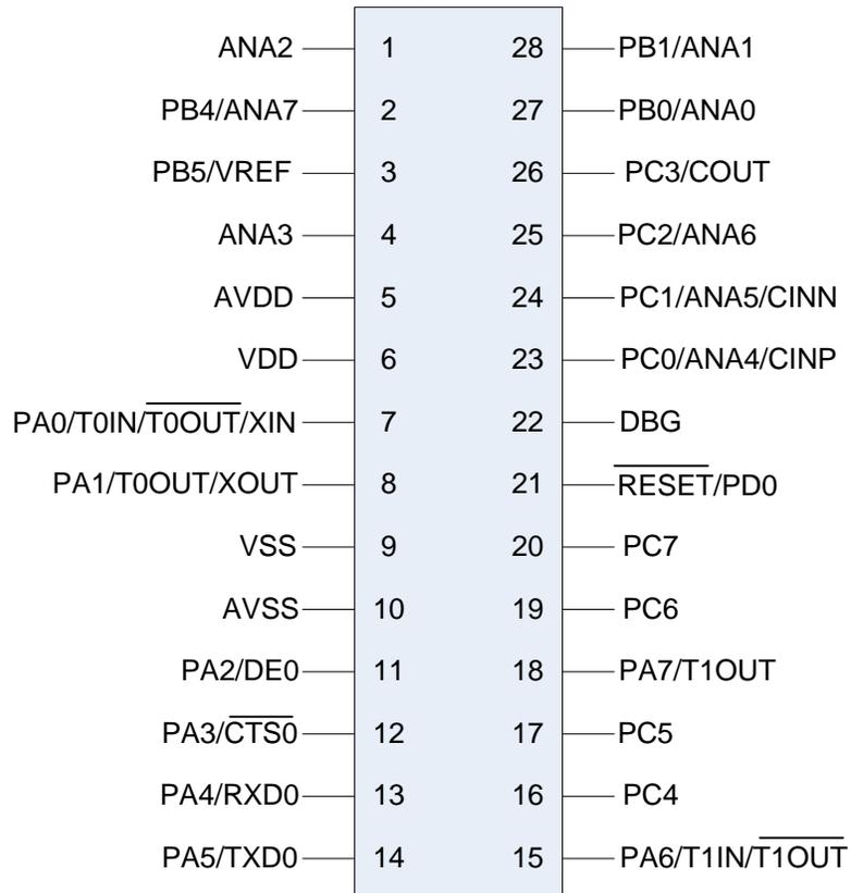
Figure 4 – 28 Pin SSOP Package Pin-Out – Z8FS040xHJ20EG
