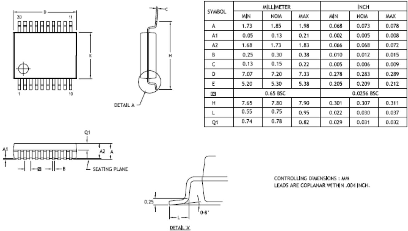
Figure 8 - 20-Pin Small Shrink Outline Package (SSOP)
