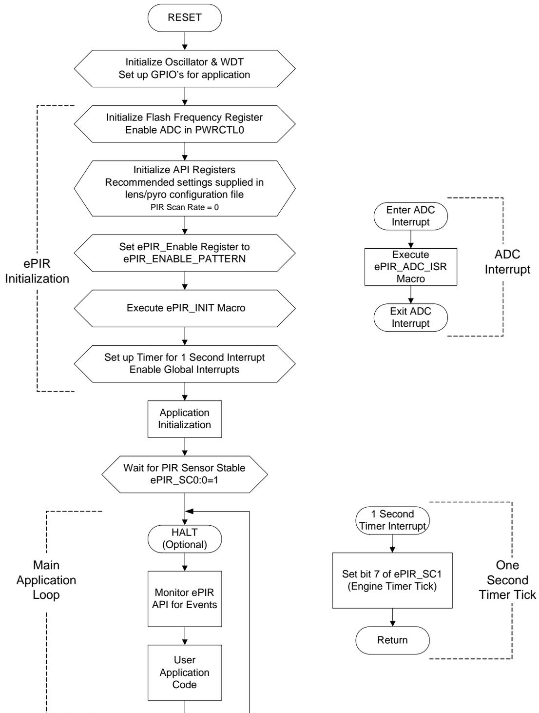
Figure 15 - Application Flow Diagram - Normal Scan Rate
