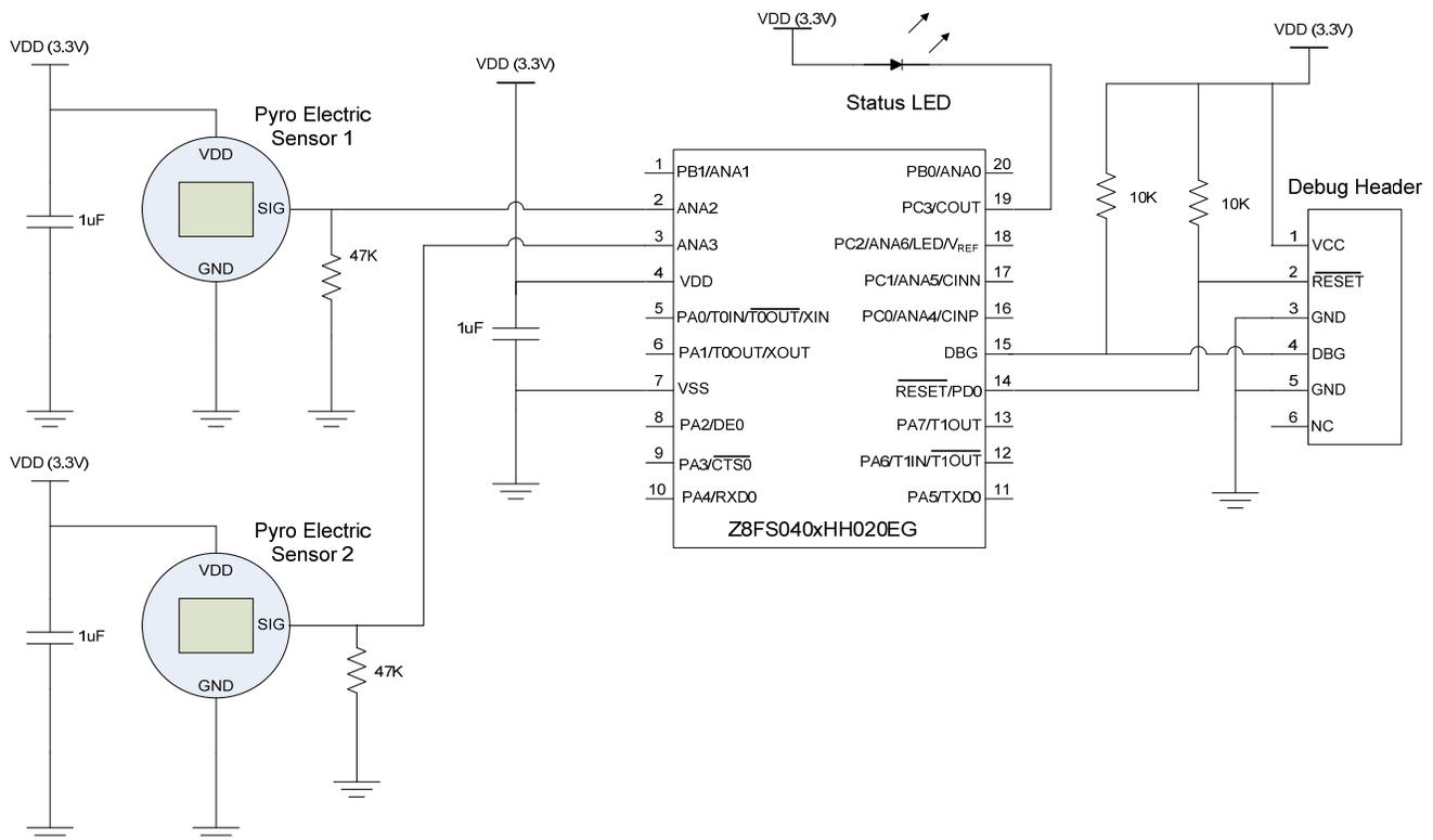
**Figure 12 - Required Circuit Connections for Z8FS040xHH020EG (20 Pin) Motion Detection MCU – Dual Pyro Mode**
