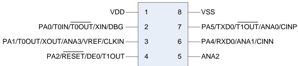
**Figure 2 – 8 Pin SOIC Package Pin-Out – Z8FS040xSB20EG**
