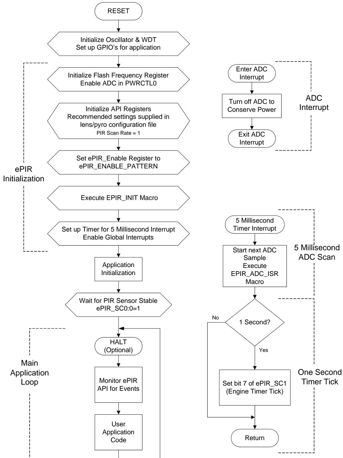
Figure 16 - Software Flow Diagram – Low Scan Mode
