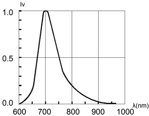
Fig. 1 Relative Luminous Intensity vs. Wavelength @ 20mA
