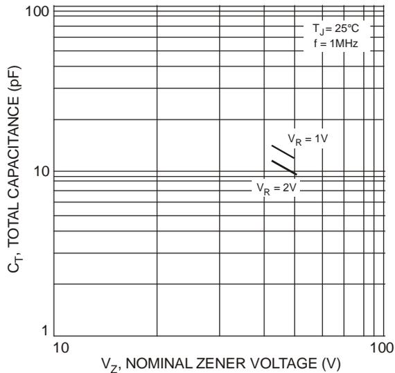
Fig. 3 Total Capacitance vs Nominal Zener Voltage
