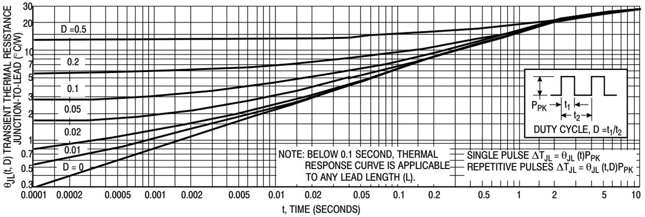
Figure 2. Typical Thermal Response L, Lead Length = 3/8 Inch
