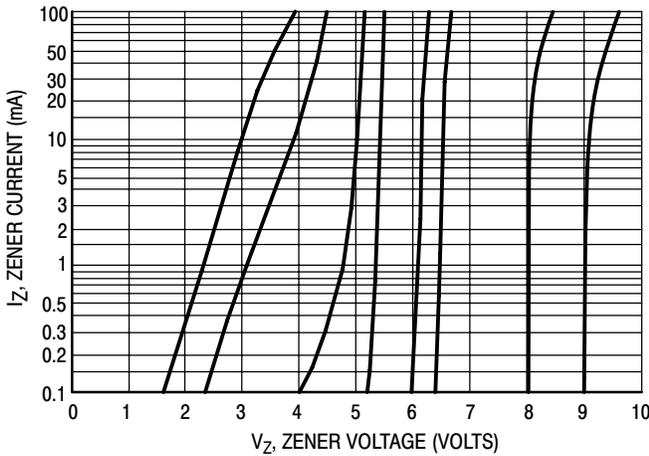
Figure 7.  $V_Z = 3.3$  thru 10 Volts
